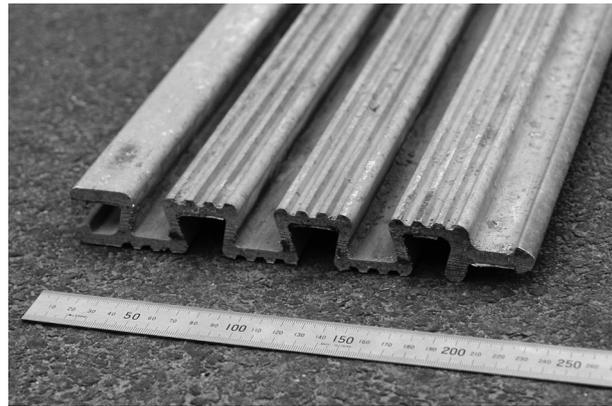
Fig. 2 Extruded aluminium section of Class 60 trackway panel
