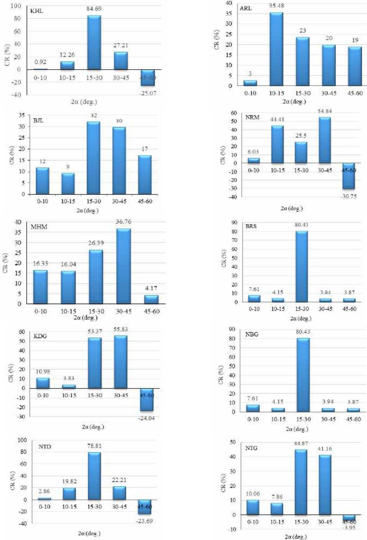
Fig. 10 Change ratio (CR) diagrams of Brazilian tensile strength with increasing  $2\alpha$  angle for the tested rock samples
