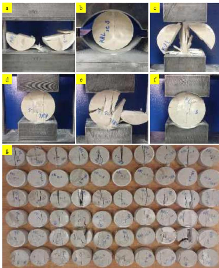
Fig. 8 Failure patterns of the sample of KHL under different  $2\alpha$  angles; (a)  $2\alpha=0^\circ$  (flat jaw), (b)  $2\alpha=10^\circ$  (standard jaw), (c)  $2\alpha=15^\circ$ , (d)  $2\alpha=30^\circ$ , (e)  $2\alpha=45^\circ$ , (f)  $2\alpha=60^\circ$  and (g) all specimens
