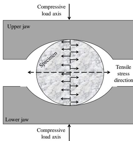
Fig. 4 Tensile stress direction in Brazilian test
