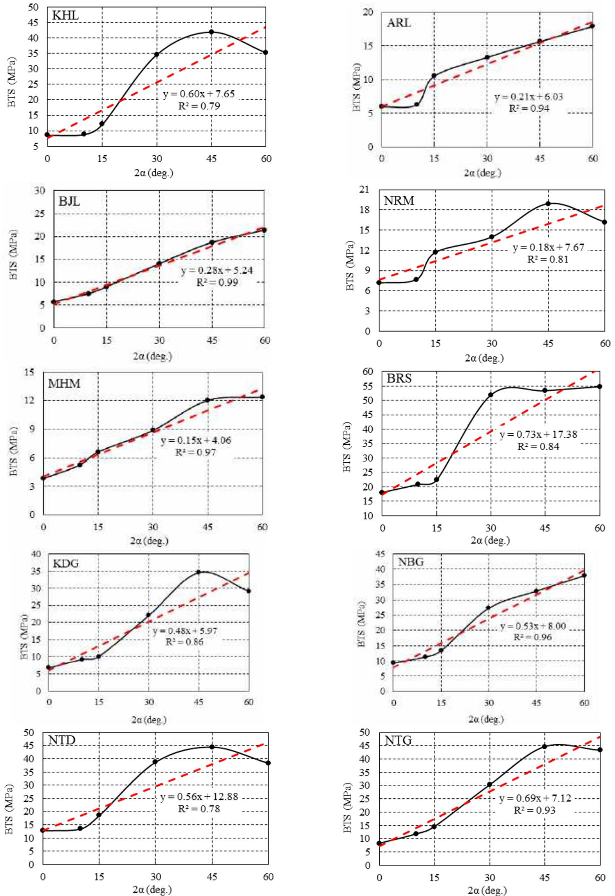
Fig. 9 Correlations between BTS and 2α angle for the tested rock samples
