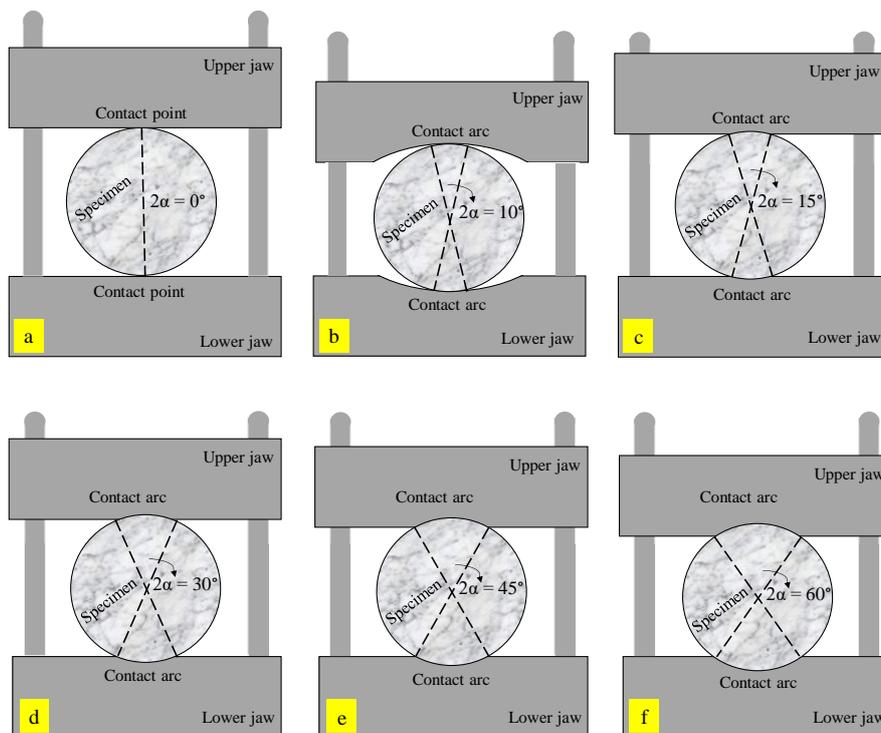
Fig. 5 Different  $2\alpha$  or contact angles in the present research; (a)  $2\alpha=0^\circ$  (flat jaw), (b)  $2\alpha=10^\circ$  (standard jaw), (c)  $2\alpha=15^\circ$ , (d)  $2\alpha=30^\circ$ , (e)  $2\alpha=45^\circ$  and (f)  $2\alpha=60^\circ$
