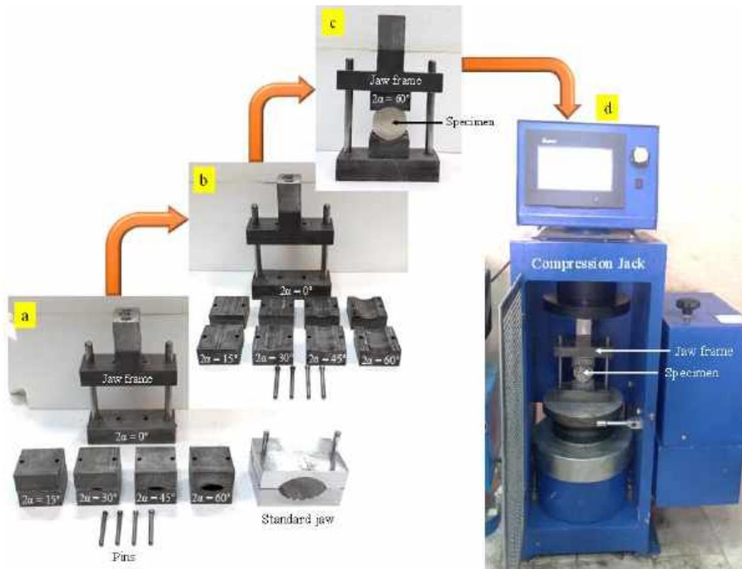
Fig. 6 Brazilian tensile strength test apparatus and its performance process in this research; (a) and (b) built Brazilian jaws from MO40 steel in different contact angles and its comparison to standard jaw, (c) placement specimen into jaws and (d) insert jaw frame containing specimen into test machine
