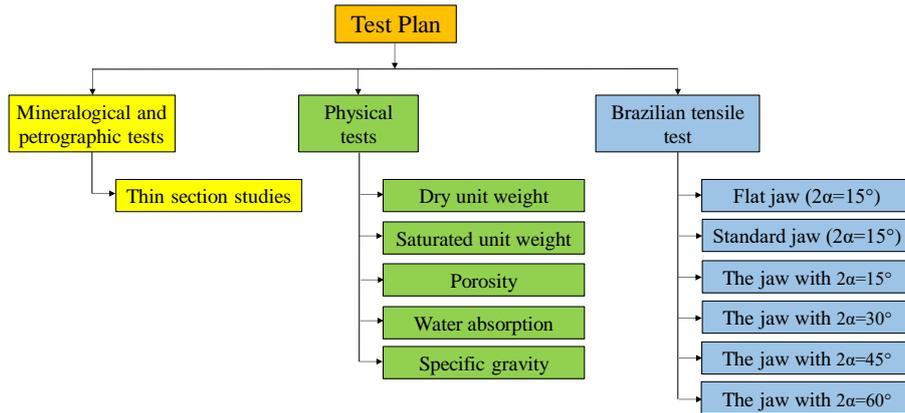
Fig. 3 Test plan for mineralogical and petrographic, physical, and Brazilian tensile tests
