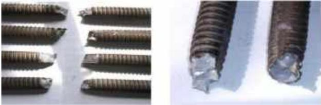
Fig. 5 Fracture surface of tensile broke bolts
