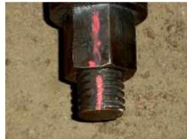
Fig. 7 The nut status when the bolt load was 300 kN
