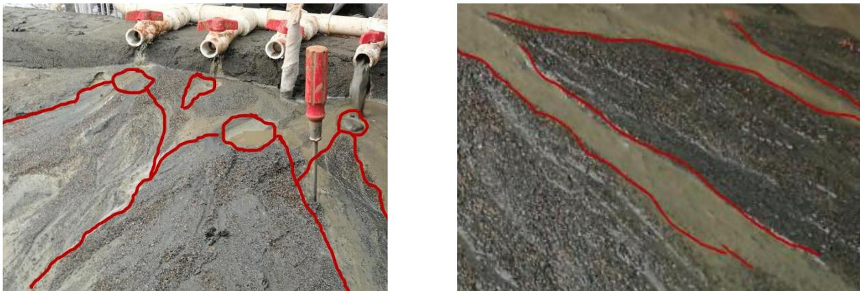
(a) Tailings pulp fan-shaped diffusion (b) Groove channel on the deposited beach surface
