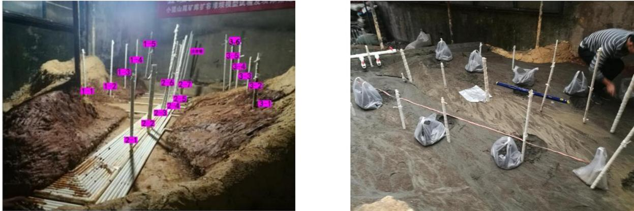
(a) Groundwater level measuring system and infiltration system (b) Sampling on the dry beach surface of the damming model system
