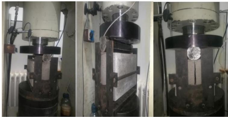
Fig. 5 Splitting test of the concrete slab
