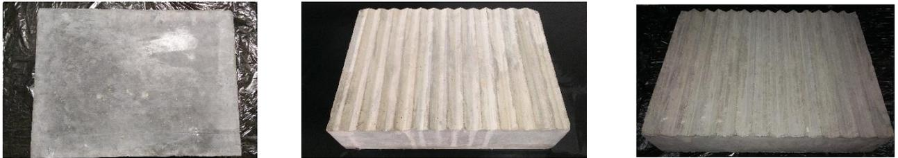
(a) Group A - 0° climbing angle concrete slab (b) Group B - 20° climbing angle concrete slab (c) Group C - 30° climbing angle concrete slab
