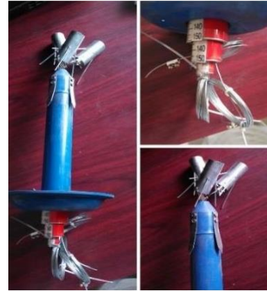
Fig. 4 The 3-point roof separation indicators
