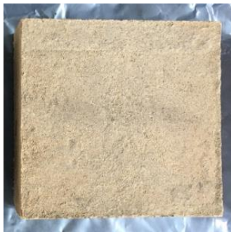
Fig. 1 The picture of the similar formed roof (Its dimensions are 0.25 m × 0.25 m × 0.07 m)
