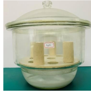
Fig. 2 A desiccator with a saturated NaCl solution
