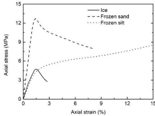
Fig. 7 Representative stress-strain curves of ice, sand, and silt frozen at -10°C
