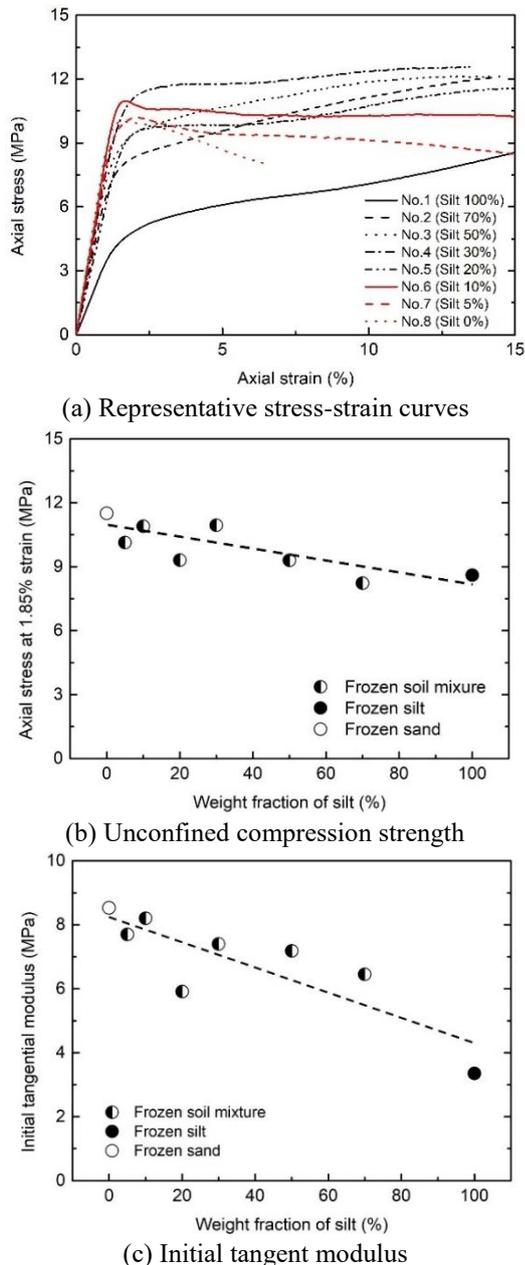
Fig. 9 Results for frozen soil mixtures at  $-10^{\circ}\text{C}$
