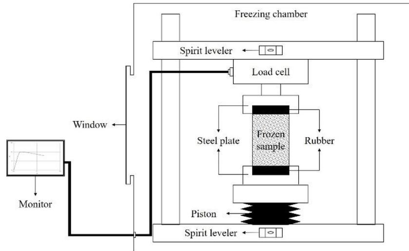
Fig. 3 Schematic diagram of equipment for unconfined compression test
