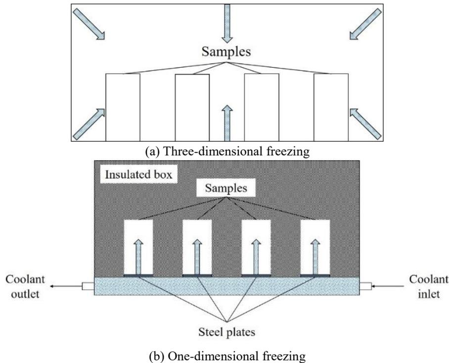
Fig. 1 Schematic diagram of frozen sample maker
