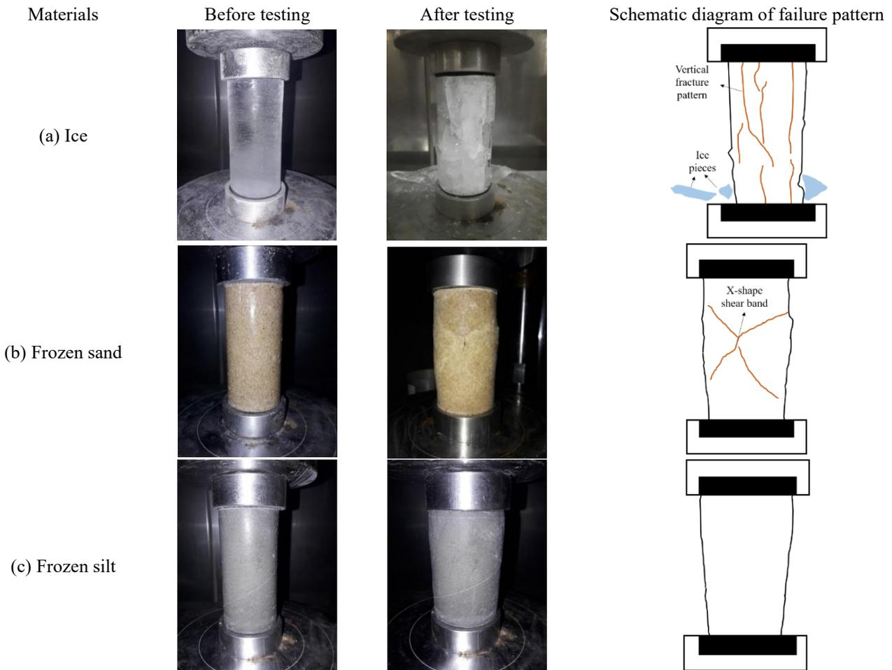
Fig. 8 Schematic diagram of failure patterns of frozen materials under unconfined compression
