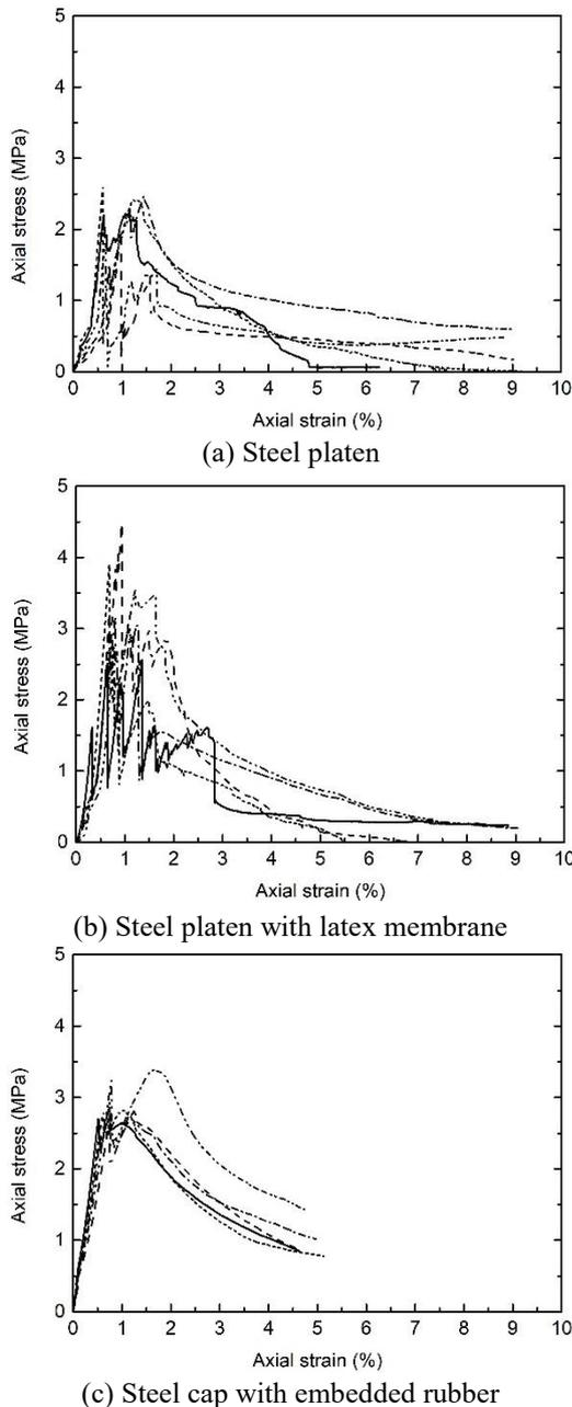
Fig. 5 Stress-strain relationships recorded at  $-10^{\circ}\text{C}$  under three different end-surface conditions
