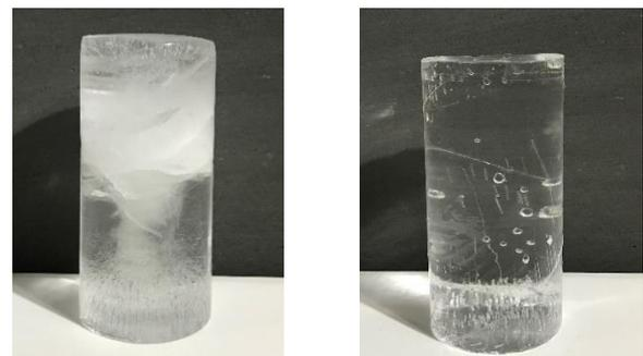
(a) Samples created by a flexible cylindrical paper mold
