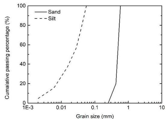
Fig. 6 Grain size distributions of sand and silt
