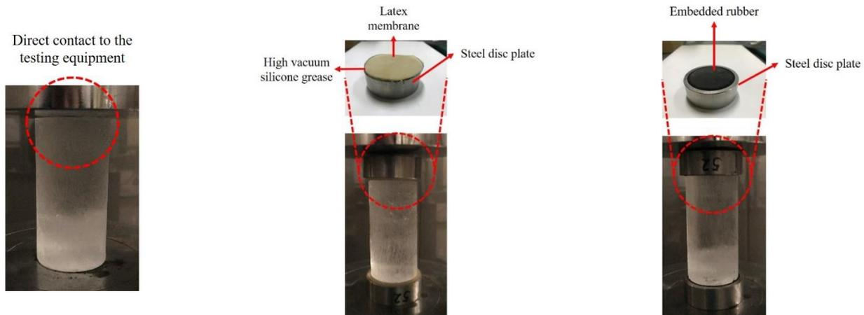
(a) Direct contact with loading plate (b) Steel disc cap with latex membrane applied high vacuum silicone grease (c) Steel disc cap with embedded rubber
