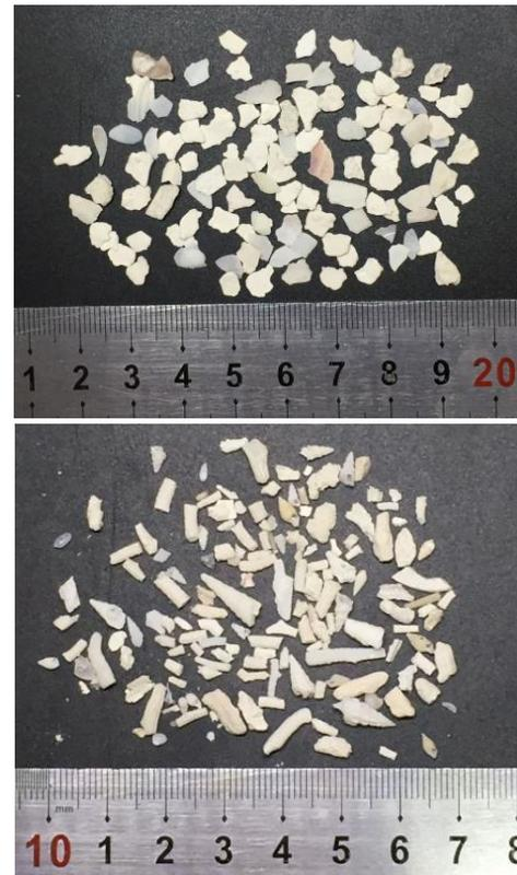
Fig. 8 Calcareous sand grains with different shapes (a) flaky and (b) long columnar
