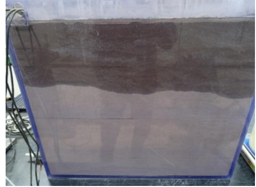
(b) Saturation condition due to rainfall infiltration
