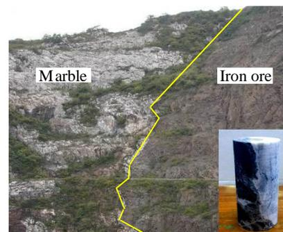
Fig. 1 Contact zone composite rock mass and composite rock sample
