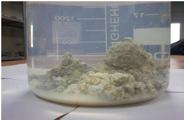
Fig. 9 Result of immersion test in upheaval zone of tunnel
