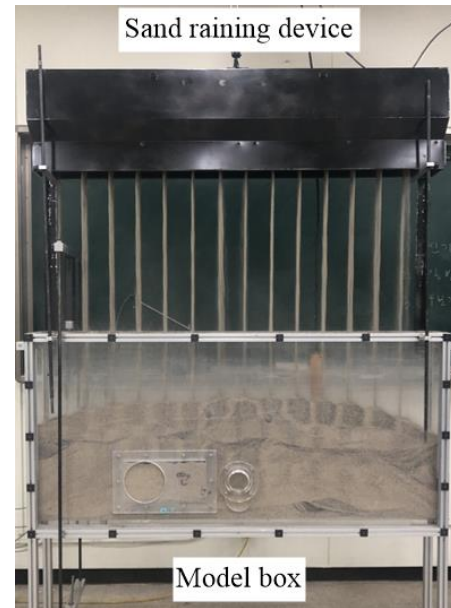
Fig. 2 Model box and sand raining device
