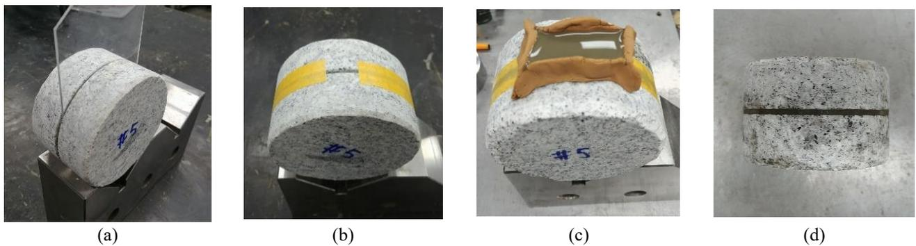
Fig. 7 Preparation of rock specimen with grout infilled (a) securing a space for grout, (b) wrapping the perimeter of the specimens, (c) building the clay inlet for allowing grout mixture infiltration and (d) removal of clay inlet and curing
