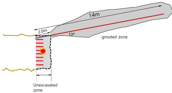
Fig. 2 Cross-sectional view of MTG
