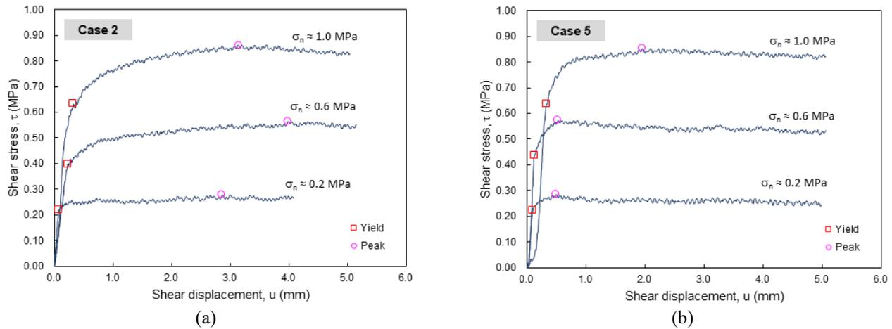
Fig. 8 Shear displacement and stress curves for cases 2 and 5 (a) case 2 and (b) case 5
