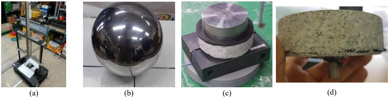
Fig. 4 Weight release system to reproduce the blasting induced vibration (a) Drop Table, (b) Steel ball, (c) Upper and bottom covers and (d) Accelerometer attached at the bottom of the rock specimen
