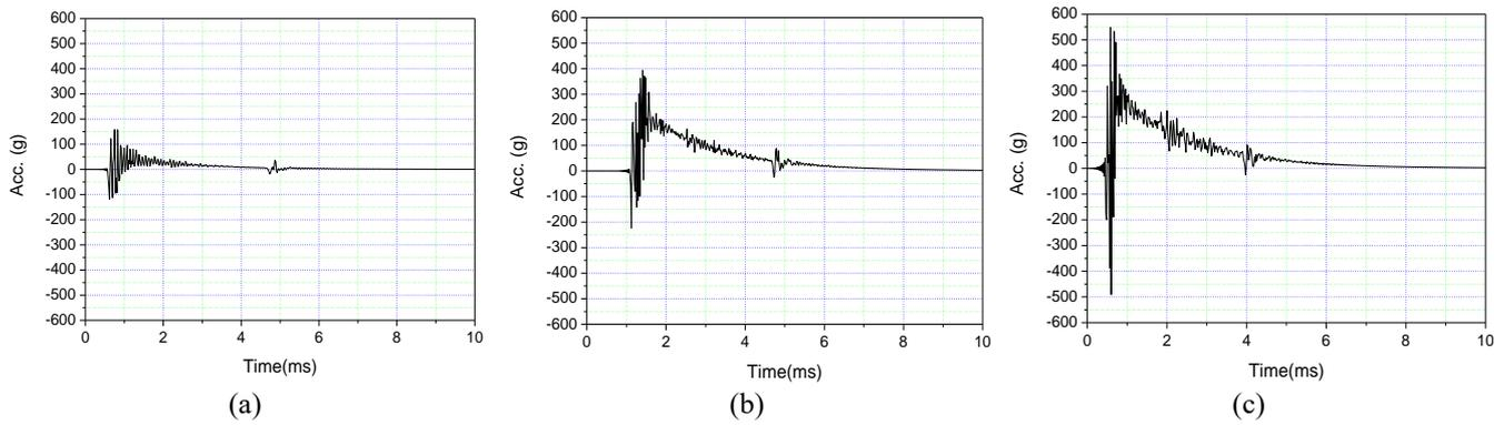
Fig. 6 Acceleration wave profile at the different heights (a) height of 10 cm, (b) height of 20 cm and (c) height of 30 cm
