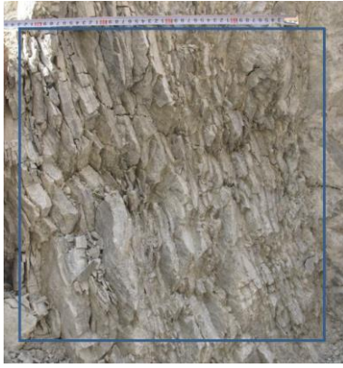
(a) Natural sample with normal stress of 0.61 MPa
