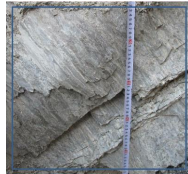
(c) Saturated sample with normal stress of 0.91 MPa
