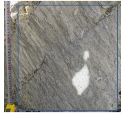
(b) Saturated sample with normal stress of 0.60 MPa
