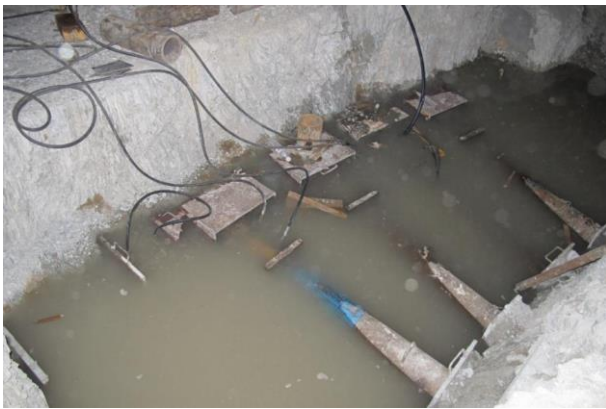
Fig. 3 Rock mass samples soaked in water for 48h
