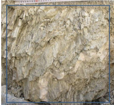
(b) Saturated sample with normal stress of 0.23 MPa
