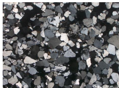
Fig. 1 Thin section image of Postaer sandstone
