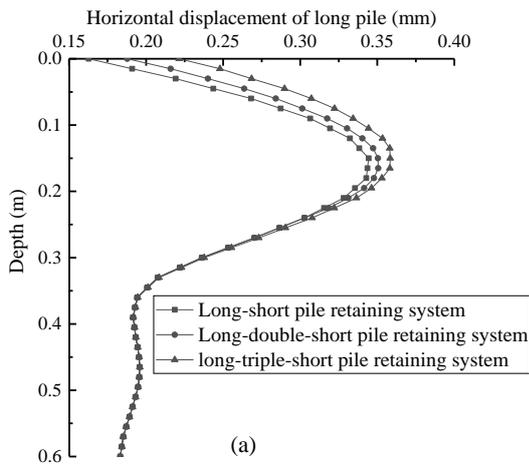
(a) The horizontal displacement of long pile
