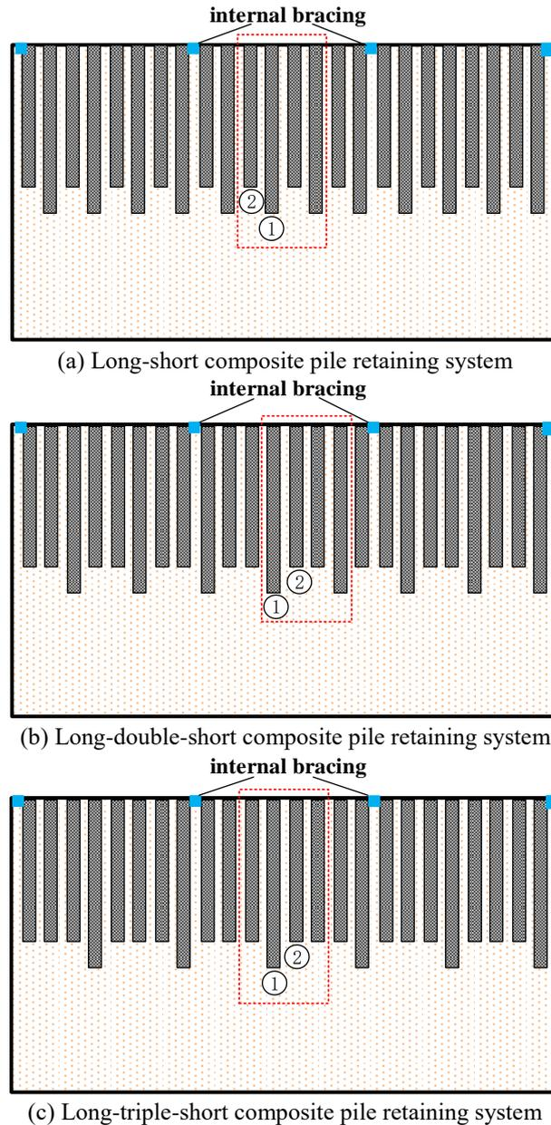
Fig. 4 Three different composite pile retaining systems
