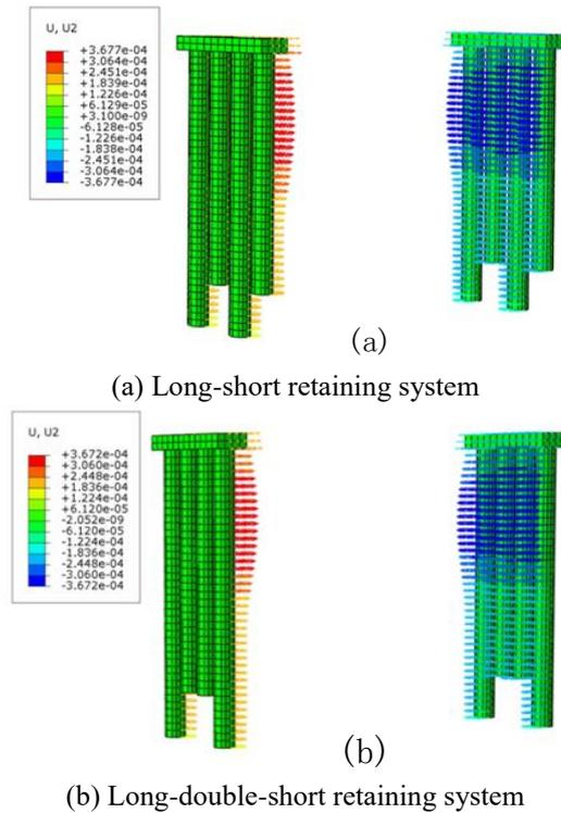
Fig. 9 Cloud picture of displacement and various curve of depth horizontal displacement
