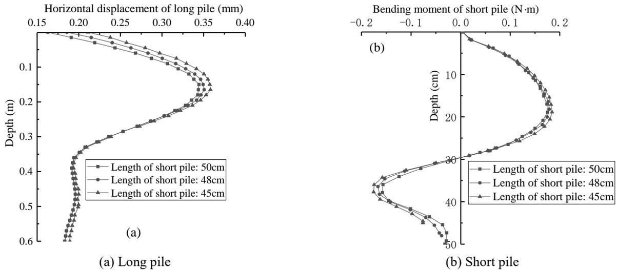
Fig. 13 Horizontal displacement distribution curves of long and short piles along different depths corresponding to the retaining system combined with short pile with different lengths and long piles with a constant length of 60 cm
