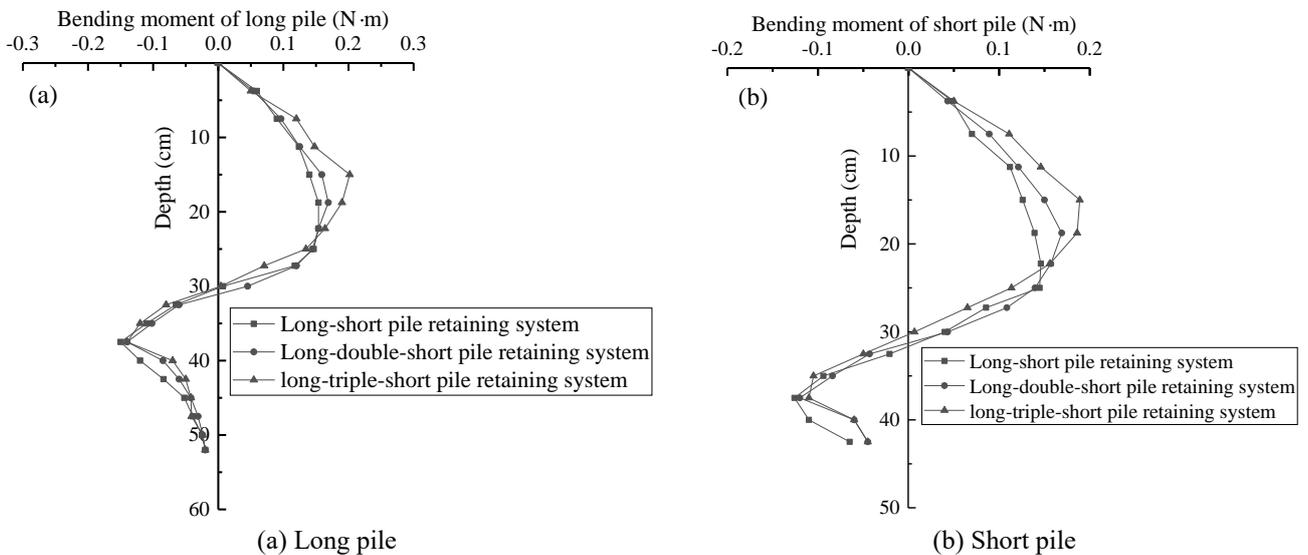
Fig. 6 Distribution curves of bending moment of piles with different long-short piles combination
