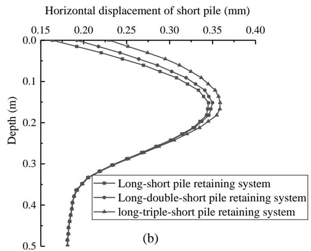
(b) The horizontal displacement of short pile
