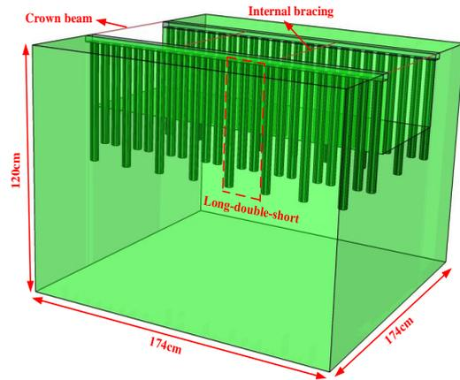
Fig. 7 Long-double-short finite element model schematic diagram
