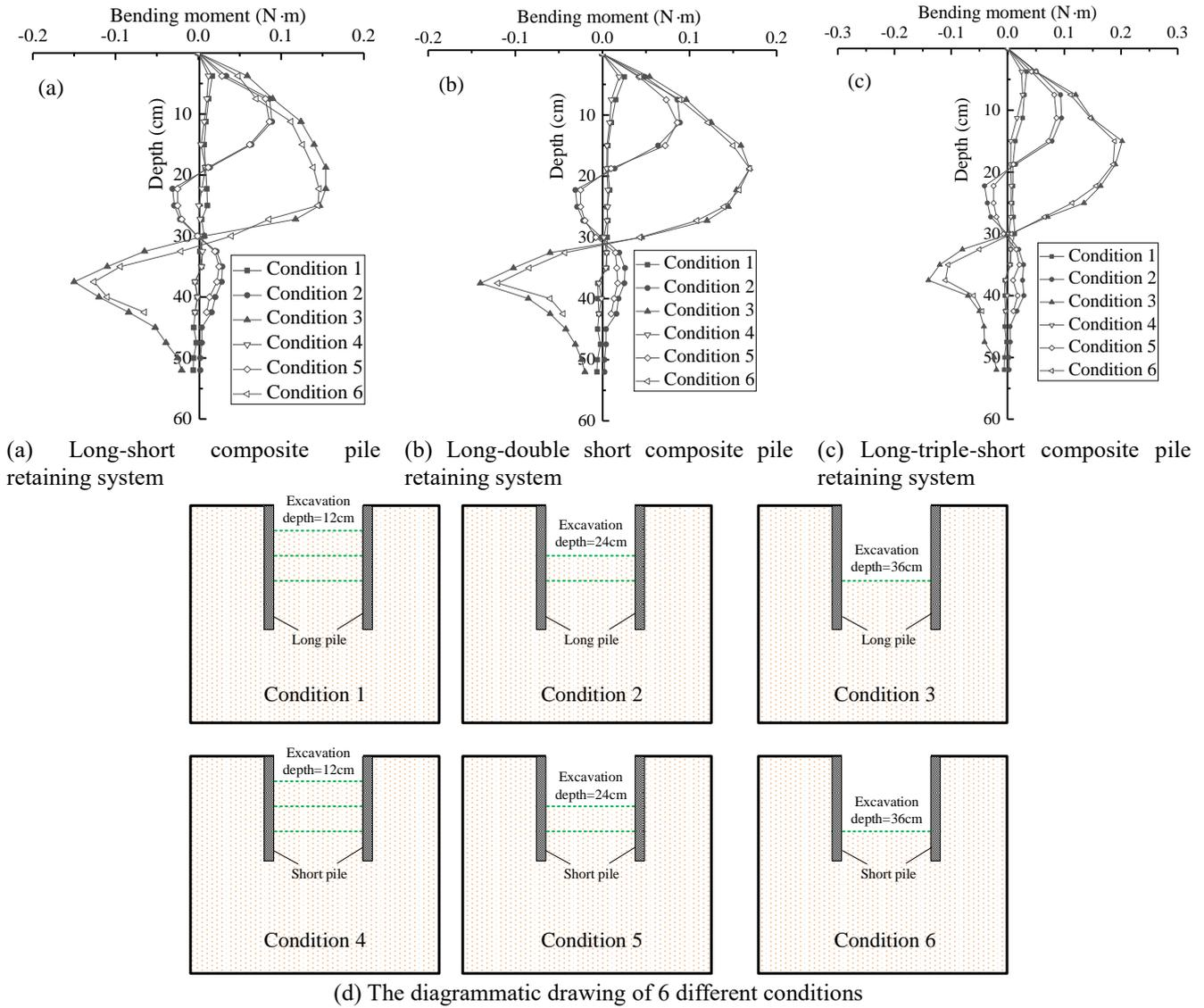
Fig. 5 Variation of the bending moment along the depth of the long and short piles, respectively, corresponding to the retaining systems with different combinations of long and short pile at different excavation stages
