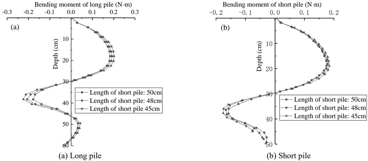
Fig. 12 Bending moment distribution curves of long and short piles along different depths corresponding to the retaining system combined with short piles with different lengths and long piles with a constant length of 60 cm
