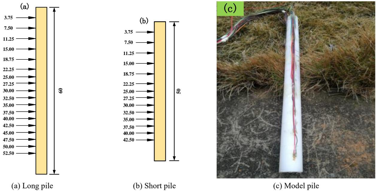
Fig. 2 Model piles and measuring point diagram (unit: cm)
