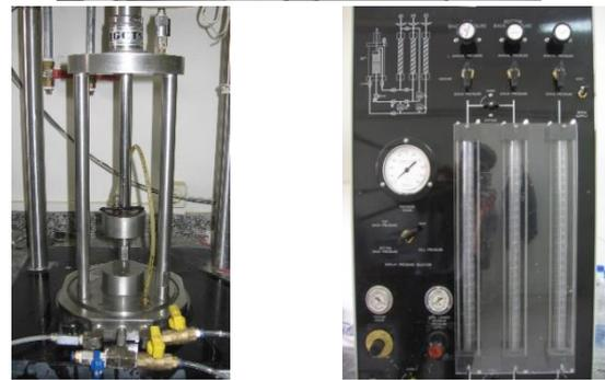
Fig. 5 GCTS triaxial apparatus used in the study
