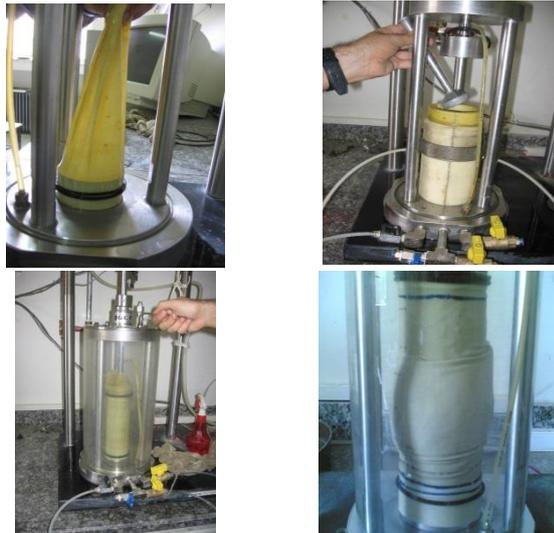
Fig. 6 Preparing sample and running triaxial test
