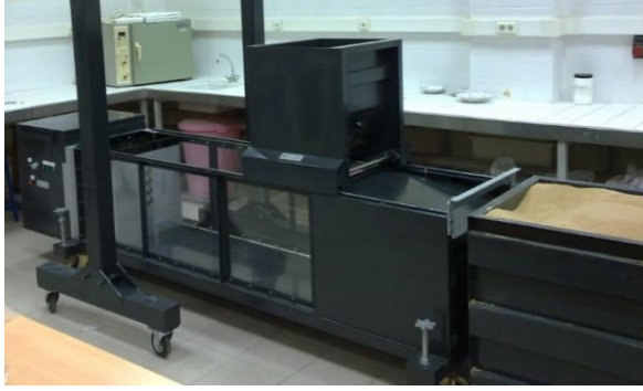
(a) Photograph of the setup with the pluviation and data acquisition systems
