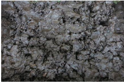
Fig. 2 Fibrous peat with water content of 495% (before consolidation process)
