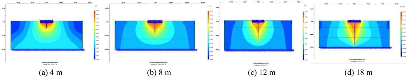
Fig. 16 The settlement of six-floor structure in the presence of raft foundation based on a single pile with a diameter of 1 m after the application of seismic load
