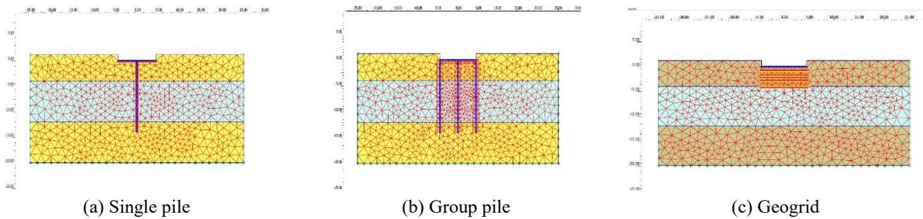
Fig. 10 Modeling for six-floor structure with (a)-(c) in different layers and lengths
