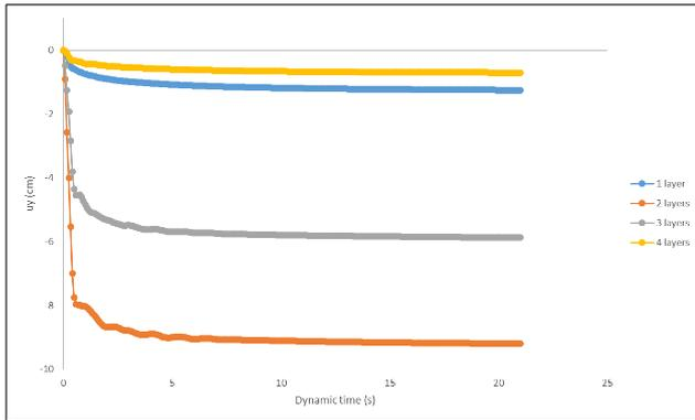
Fig. 20 Dynamic Time-Settlement graph, the effect of geogrid layering on soil settlement over a period of 21 seconds
