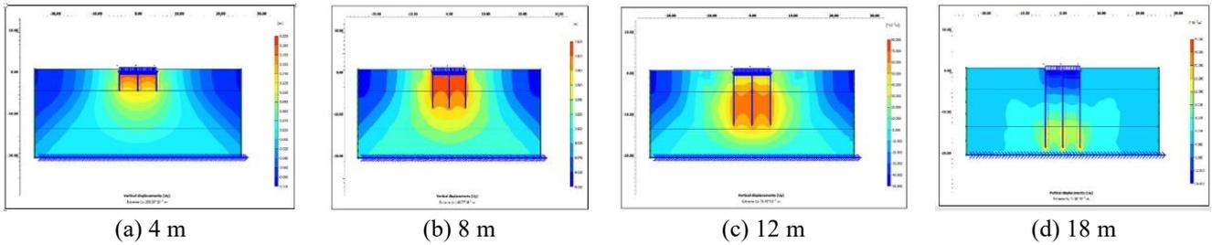
Fig. 13 The settlement of the six-floor structure in the presence of a raft foundation based on pile group with a diameter of 0.8 meter after application of the seismic load
