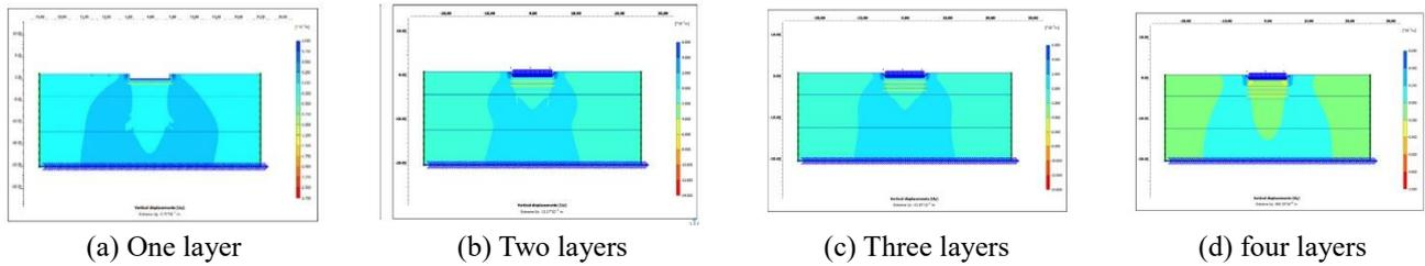
Fig. 17 The settlement of six-floor structure in the presence of geogrid after the application of seismic load
