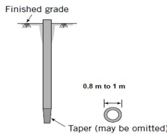
Fig. 7 Precast and pre-stressed single concrete pile with a circular cross section of different diameters (Mahmoudi Azar 2017)
