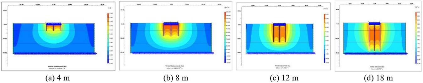
Fig. 14 The settlement of the six-floor structure in the presence of a raft foundation based on pile group with a diameter of 1 meter after application of the seismic load
