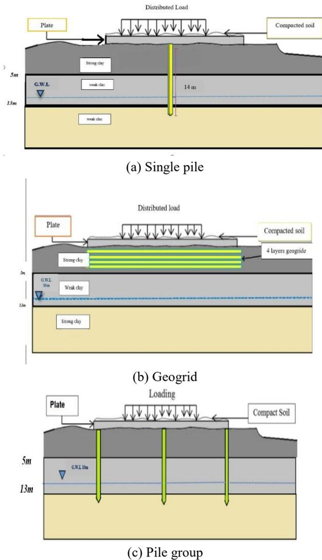
Fig. 8 Geotechnical models of the soil profile of the studied area in the presence of (a)-(c) (Mahmoudi Azar 2017)
