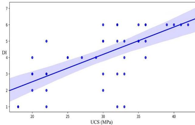
Fig. 22 Deterioration index versus UCS
