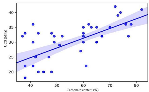
Fig. 19 UCS versus carbonate content
