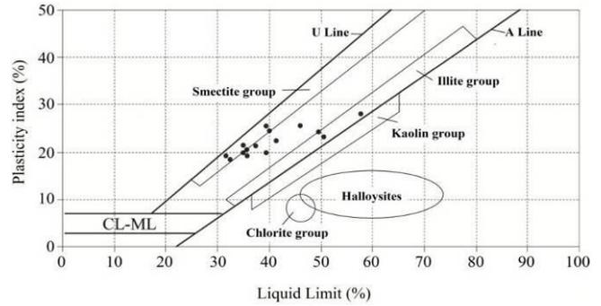
Fig. 8 Distribution of the marly soils and the clay minerals on the Holtz and Kovacs (1981) chart
