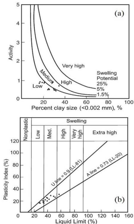
Fig. 9 SPZ marl activity according to: (a) Skempton chart and (b) Seed *et al.* chart (from Yilmaz 2006)
