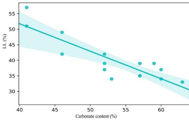
Fig. 14 Liquid limit versus carbonate content
