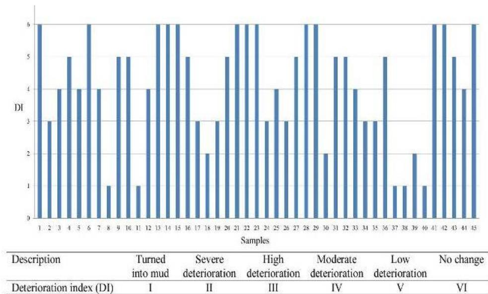
Fig. 11 Durability test results and deterioration index (DI) of the SPZ marls
