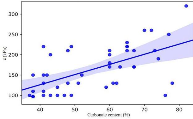
Fig. 20 Cohesion versus carbonate content
