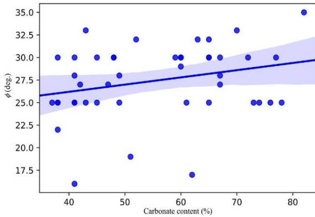
Fig. 21 Friction angle versus carbonate content
