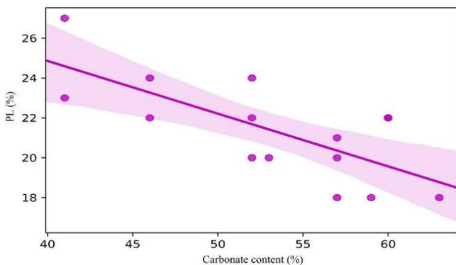
Fig. 15 Plasticity limit versus carbonate content
