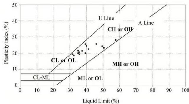
Fig. 7 The plasticity of the samples on the Casagrande chart
