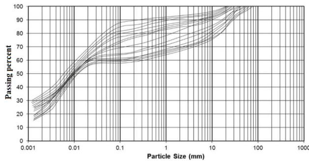
Fig. 6 The particle-size distribution and hydrometer test results of the SPZ marls
