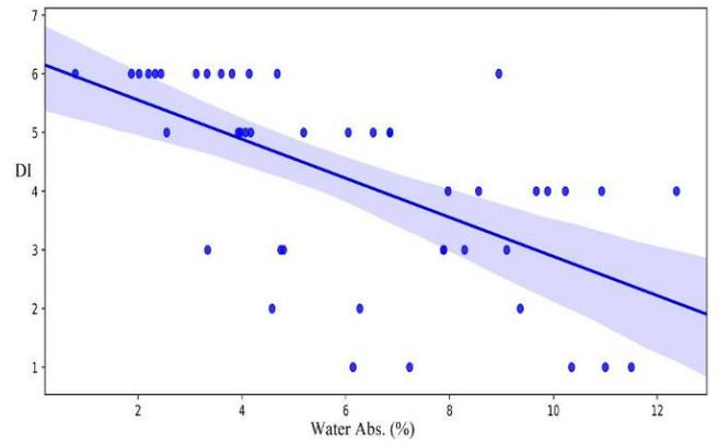
Fig. 17 Deterioration index versus water absorption
