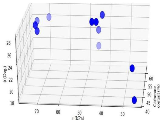
Fig. 26 Deterioration index vs. strength parameters of the SPZ marls
