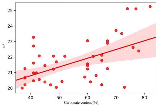
Fig. 13  $\gamma_d$  (kN/m<sup>3</sup>) variation versus carbonate content
