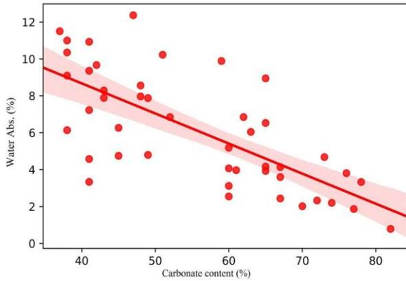
Fig. 12 Relationship between water absorption variation and carbonate content
