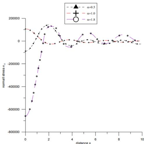
Fig. 18 Variation of normal stress  $\sigma_{33}$  with distance  $x$  uniformly distributed thermal source)
