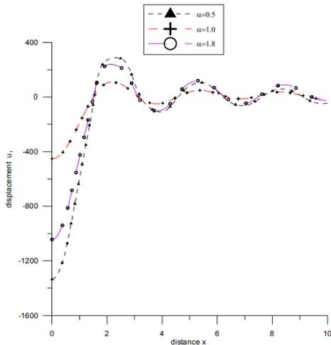
Fig. 16 Variation of tangential displacement  $u$  with distance  $x$  (uniformly distributed thermal force)
