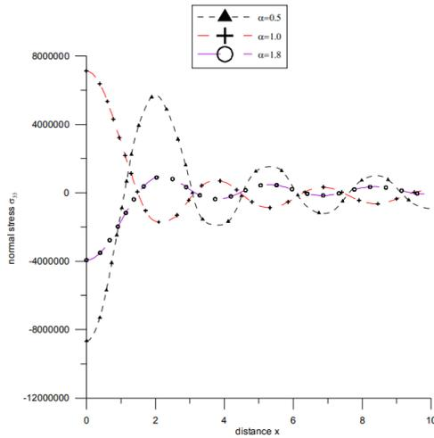
Fig. 13 Variation of normal stress  $\sigma_{33}$  with distance  $x$  (concentrated thermal Source)
