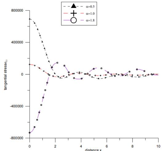
Fig. 20 Variation of tangential stress  $\sigma_{33}$  with distance  $x$  (uniformly distributed thermal source))
