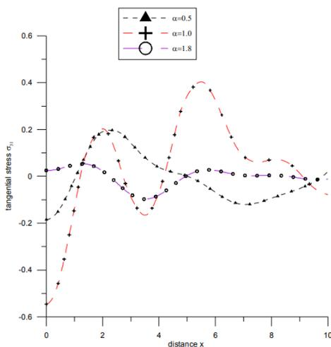
Fig. 15 Variation of tangential stress  $\sigma_{31}$  with distance  $x$  (concentrated thermal source)
