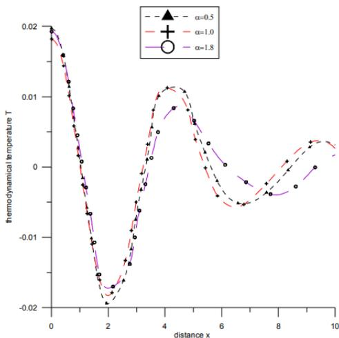
Fig. 9 Variation of temperature change  $T$  with distance  $x$  (uniformly distributed mechanical force)
