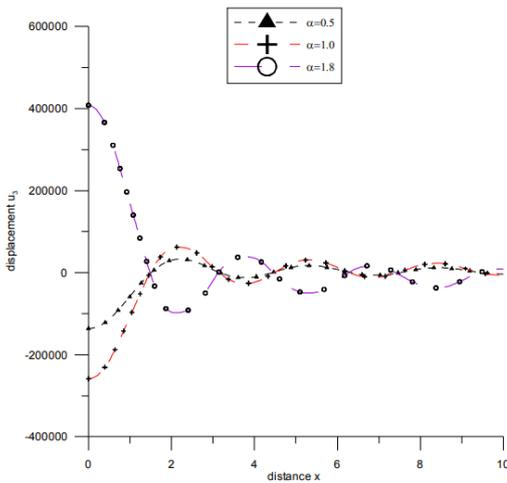
Fig. 12 Variation of normal displacement  $w$  with distance  $x$  (concentrated thermal source)
