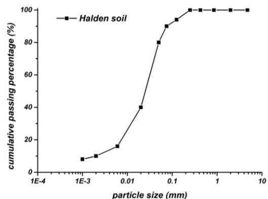
Fig. 2 Grain size distribution curve of Halden soil
