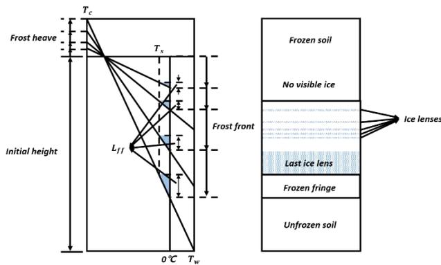
Fig. 1 Schematic diagram of frozen soil under constant temperature condition at the surface (Konrad and Morgenstern 1980) ▽ : frozen fringe
