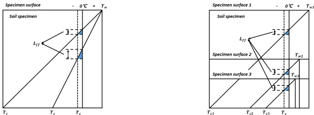
(a) Different frozen fringe thicknesses ( $L_{ff}$ ) at steady state temperatures
