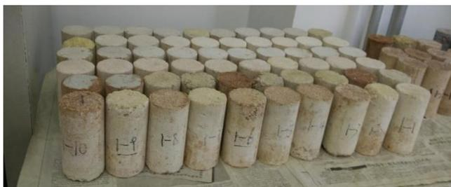
Fig. 4 Cylindrical specimens
