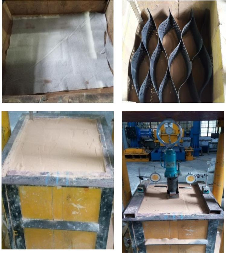
Fig. 7 Setup for plate load test in the present study
