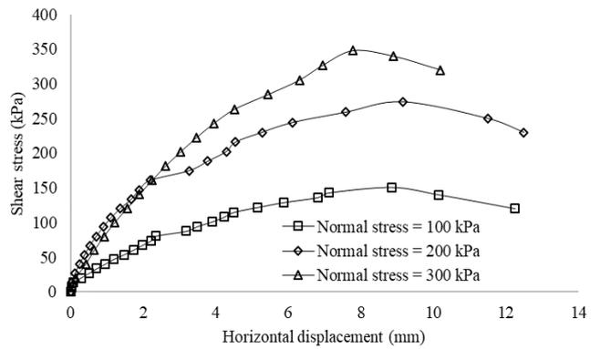
Fig. 10 Shear stress vs horizontal displacement for geocell reinforced soil
