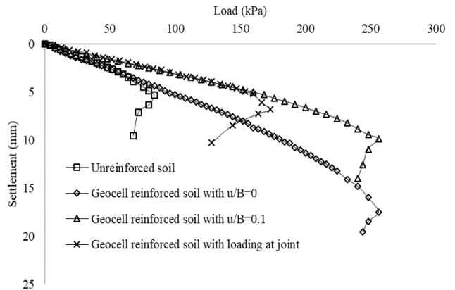
Fig. 11 Load vs settlement curve obtained from plate load test
