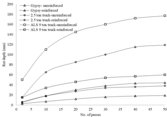
Fig. 12 Rut depth vs no. of passes in unreinforced and geocell reinforced soil
