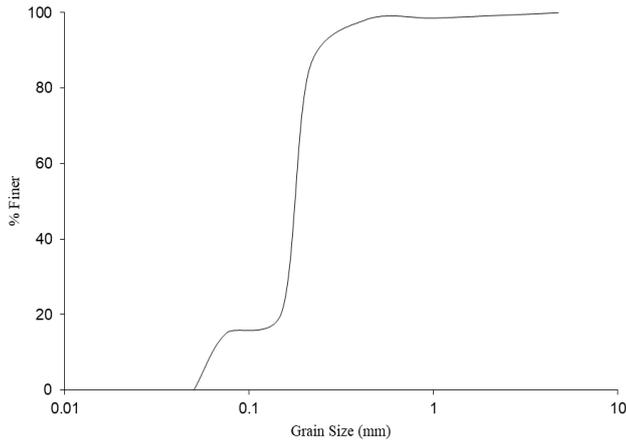
Fig. 3 Grain size distribution curve
