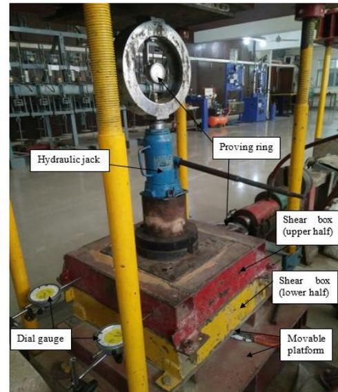
Fig. 4 Setup of direct shear test
