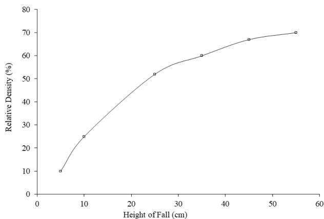
Fig. 6 Calibration curve for relative density of sand using pluviation technique
