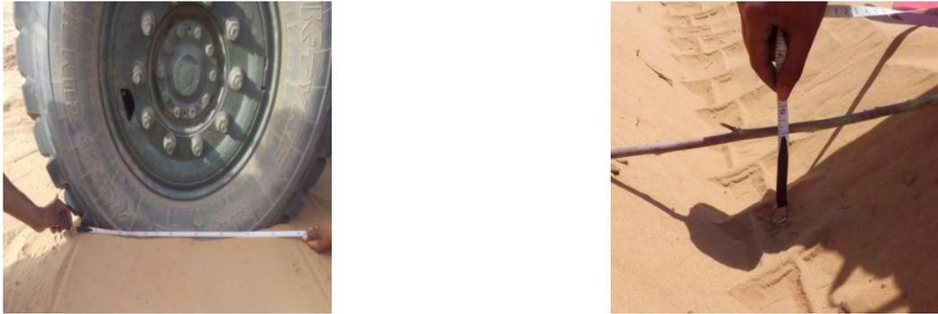
Fig. 2 Measurements of rut depth during field tests
