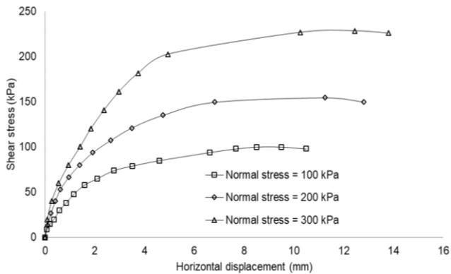
Fig. 9 Shear stress vs horizontal displacement for unreinforced soil
