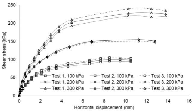
Fig. 8 Three repeated results for each vertical load showing shear stress vs horizontal displacement for unreinforced soil in direct shear test
