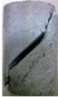
(b) Prefabricated crack of 30° inclination
