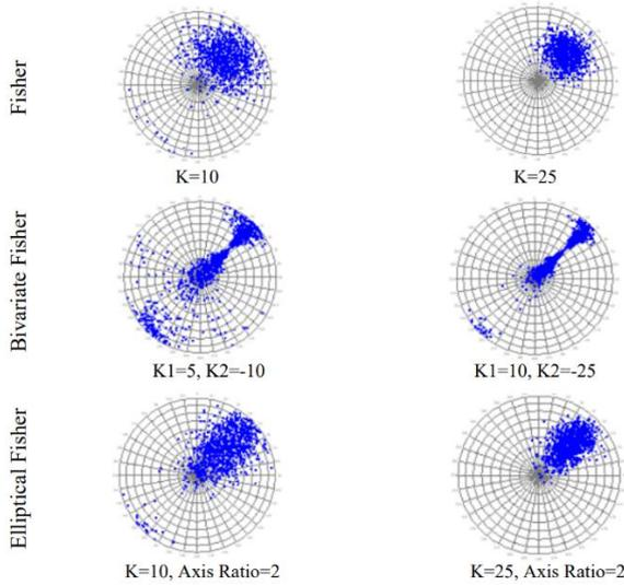
Fig. 8 Distribution of fracture orientation based on Fisher's K value
