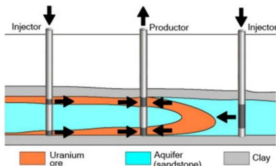
Fig. 1 In-situ leaching system (Pokalai *et al.* 2016)
