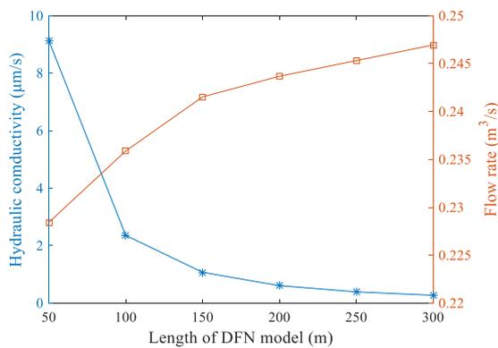
Fig. 12 Variation of hydraulic conductivity and flow rate versus DFNs model size
