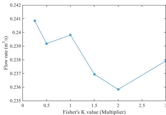
Fig. 13 Variation of flow rate versus natural fracture orientation
