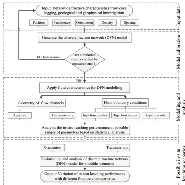
Fig. 5 Procedure for in-situ leaching simulation on pre-existing natural fractures
