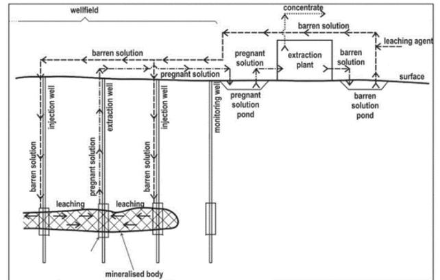
Fig. 2 The mechanism of in-situ leaching method (Sereдкиn *et al.* 2016)
