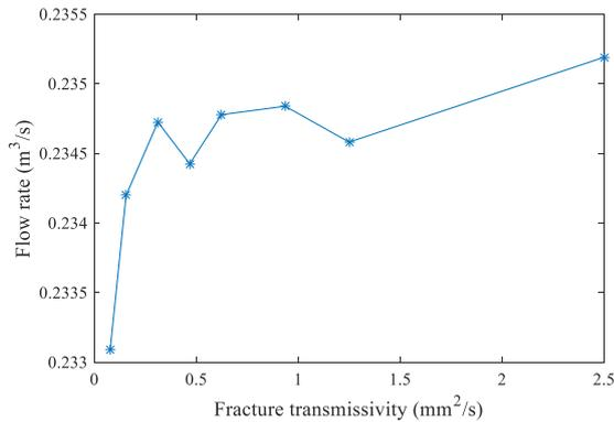
Fig. 14 Variation of flow rate versus natural fracture transmissivity
