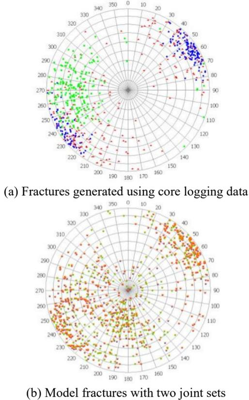
Fig. 9 The calibration of DFNs modelling
