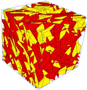
Fig. 11 Three-dimensional DFN model with two discontinuity sets
