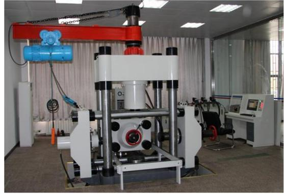
Fig. 2 Stress-seepage coupling true triaxial test system for high water pressure rock
