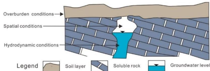
Fig. 4 Formation conditions of a karst collapse
