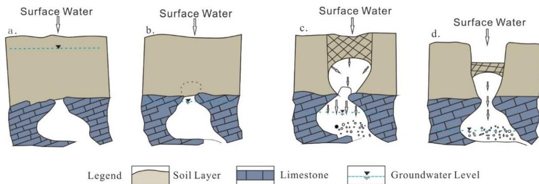
Fig. 11 The karst collapse formation process
