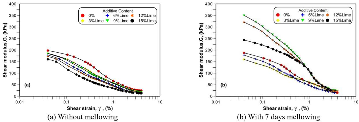
Fig. 9 Shear modulus and shear strain relationship depending on the lime content
