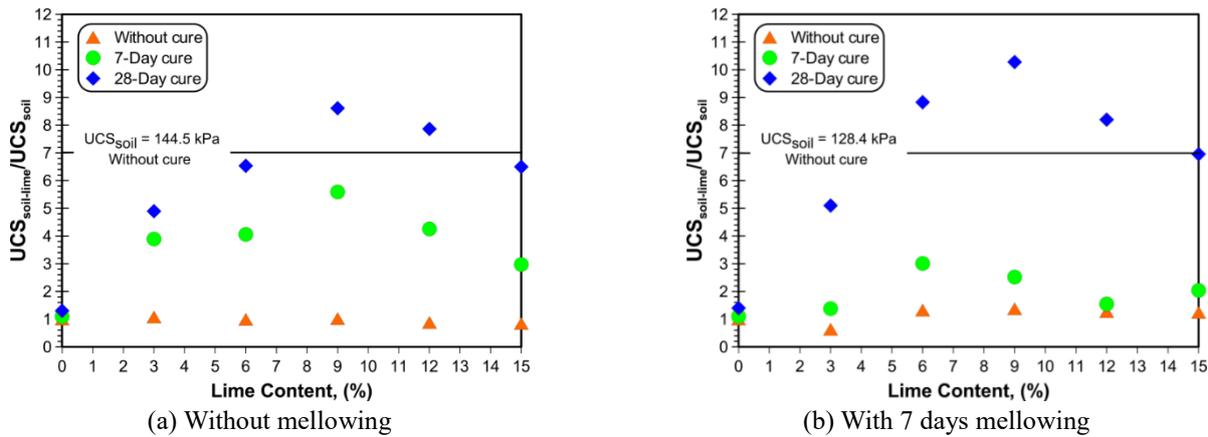
Fig. 6 Effects of lime content and curing time on UCS
