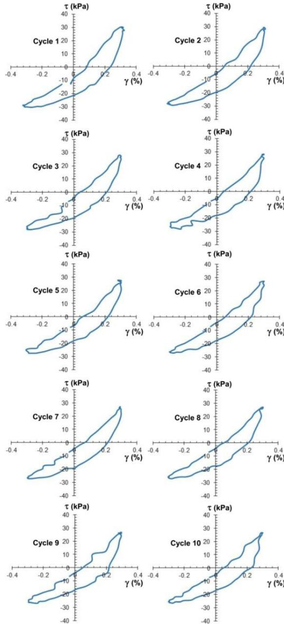
Fig. 8 Shear stress-shear strain hysteresis loops for the case of 3%lime at the 7 days mellowing period at 0.3% shear strain level
