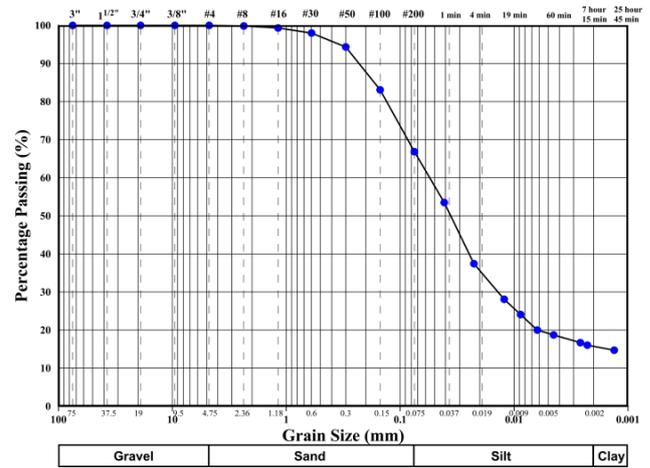
Fig. 1 The grain size distribution for the soil sample used in the study
