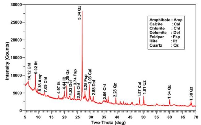
Fig. 2 XRD pattern of the soil sample
