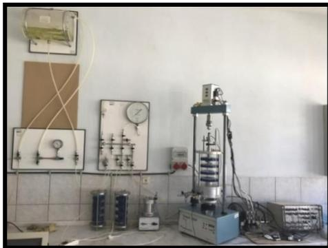
Fig. 3 Laboratory position of the dynamic triaxial testing equipment used in this study
