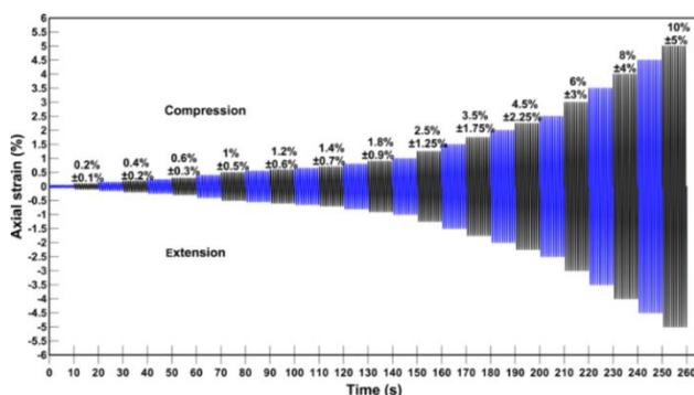
Fig. 4 Applied axial strain levels (double amplitude) during dynamic triaxial test
