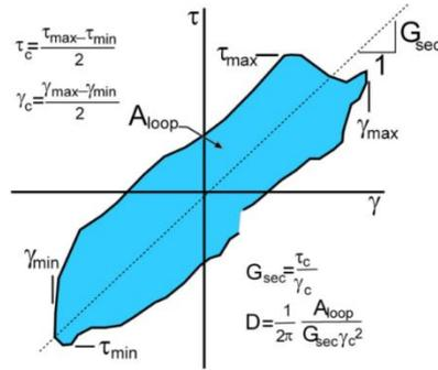
Fig. 7 An example of stress-strain loop and quantities used for evaluation of secant modulus  $G_{sec}$  and damping  $D$
