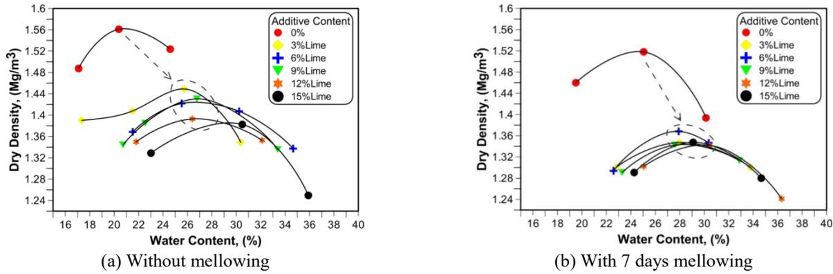
Fig. 5 Compaction curves of specimens mixed with different percentages of lime
