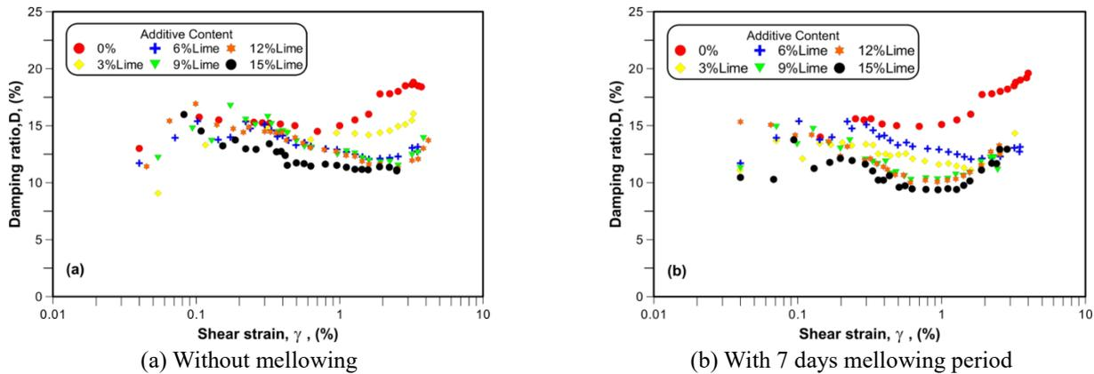
Fig. 11 Damping ratio and shear strain relationship depending on the lime content
