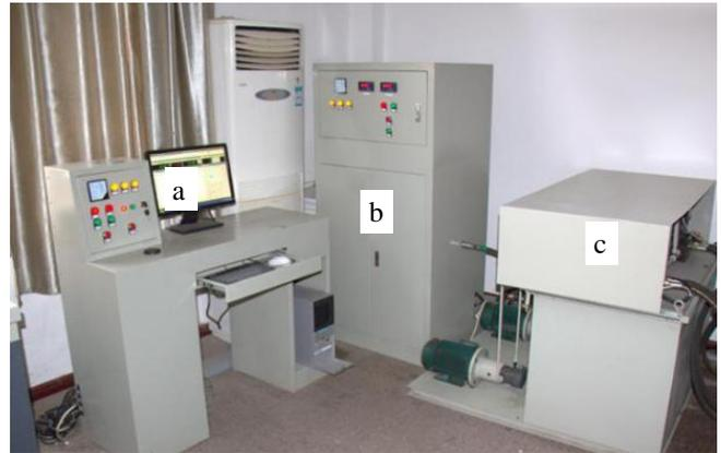
Fig. 4 Testing control system (a) Console, (b) Hydraulic pressure double control servo system and (c) Displacement stress double control servo system
