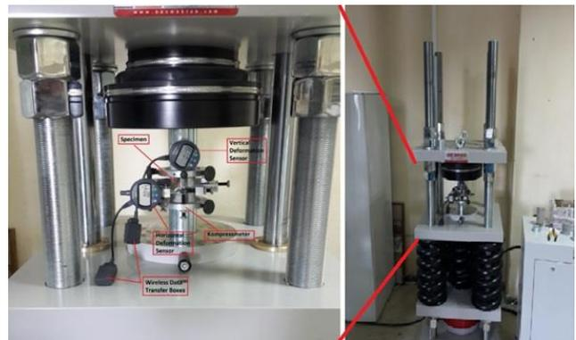
Fig. 4 Servo-controlled compressive loading press for time-dependency experiments
