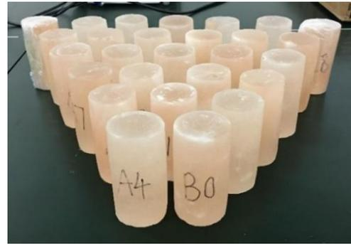
Fig. 1 Rock salt specimens
