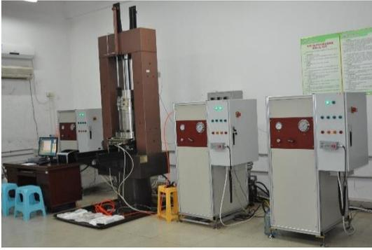
Fig. 2 TFD-2000 microcomputer servo control rock triaxial rheometer
