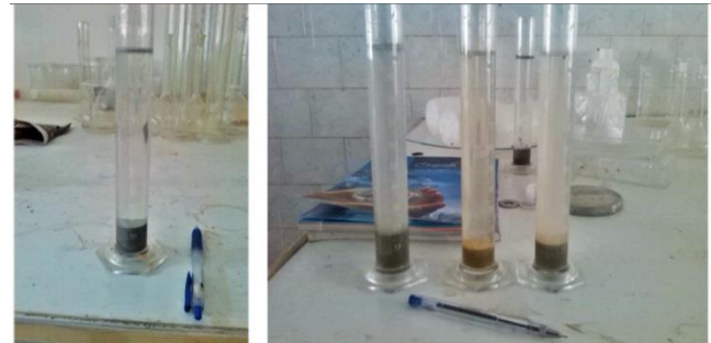
Fig. 17 Baghmisheh marls after 24 hours swelling based on Rao et al. (1987) method
