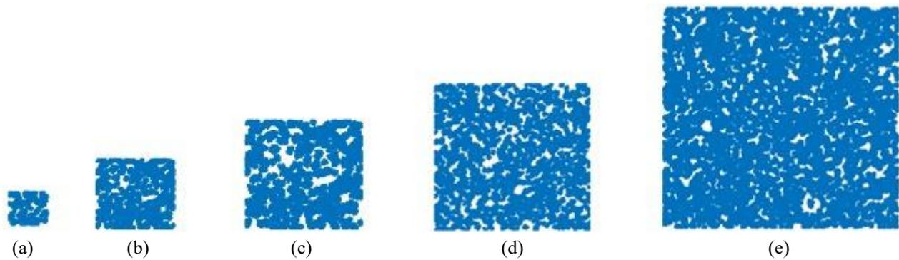
Fig. 8 Soil structures with different model sizes: (a)  $100 \times 100$ , (b)  $200 \times 200$ , (c)  $300 \times 300$ , (d)  $400 \times 400$  and (e)  $600 \times 600$
