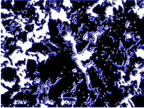
(b) DIP for calculating the properties of soil particles
