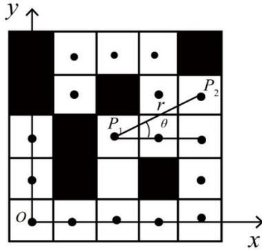
Fig. 4 Schematic diagram for estimating directional growth probability parameter ( $P_{di}$ )
