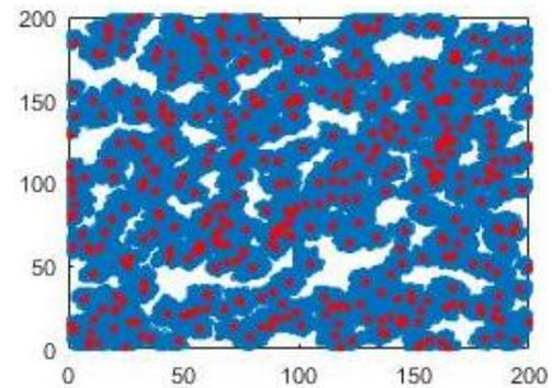
Fig. 2 A random realization of soil micro-structure ( $n_p = 0.39$ ,  $P_c = 0.01$ ,  $P_{d14} = 0.15$  and  $P_{d58} = 0.25P_{d14}$ ). The red point, the blue part, and the white part represents initial solid cores, soil particles, and pores, respectively)
