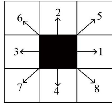
Fig. 1 Eight growth directions of a grid in 2-dimensional coordinate system
