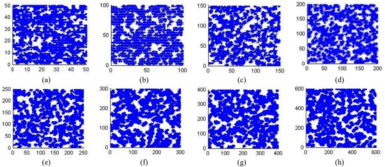
Fig. 6 Soil structures with different number of grids: (a) 50×50, (b)100×100, (c)150×150, (d)200×200, (e)250×250, (f)300×300, (g)400×400 and (h)600×600
