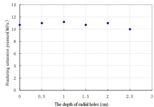
Fig. 13 The relationship between the pressures of fracture extension and the depth of radial holes
