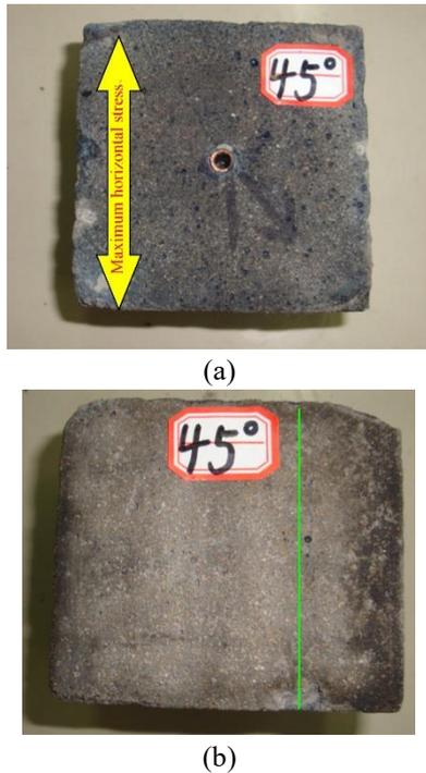
Fig. 6 Crack morphology of Sample II-3 after the test
