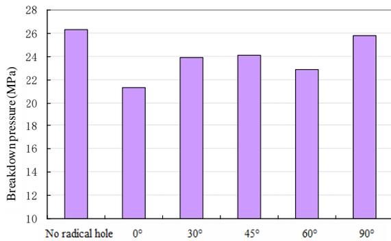
Fig. 10 The relationships between the breakdown pressures and radical hole orientations
