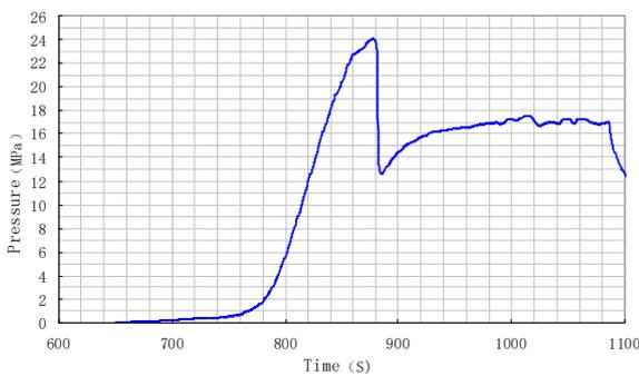
Fig. 7 Fracturing simulation curve of Sample II-3
