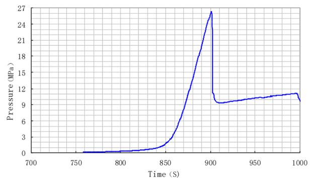
Fig. 5 Fracturing simulation curve of Sample I
