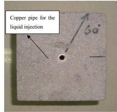
Fig. 2 Untested rock specimens after processing
