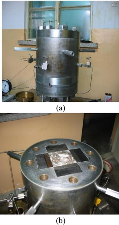
Fig. 1 The tri-axial simulation device for the hydraulic fracturing
