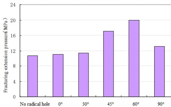
Fig. 11 The relationships between the pressures of fracture extension and radical hole orientations
