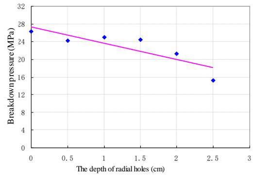
Fig. 12 The relationships between the breakdown pressures and the depth of radial holes
