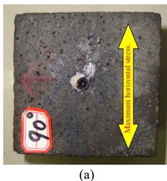
Fig. 8 Crack morphology of Sample II-5 after the test
