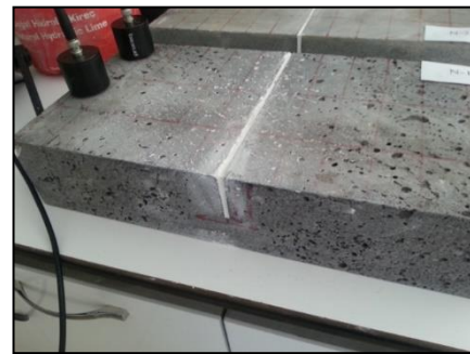
Fig. 5 The filled fracture conditions with natural hydraulic lime mortar
