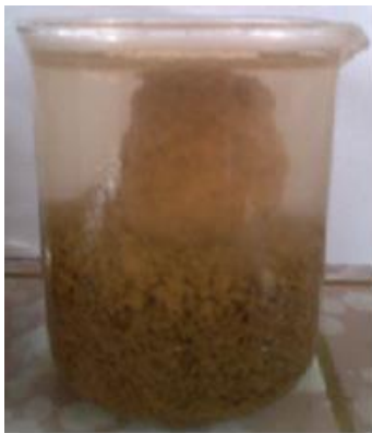
Fig. 13 The complete collapse of the untreated specimen after 30 minutes from the beginning of exposure to water
