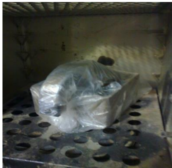
Fig. 5 Sealed specimen inside the shear box for curing
