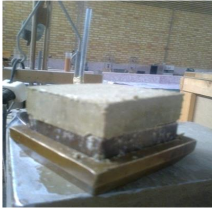
Fig. 4 Specimen extracted by surcharge from the mold
