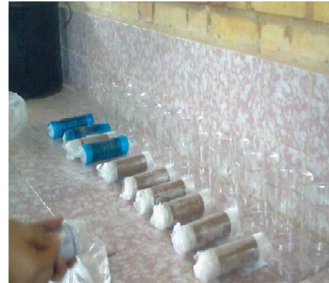
Fig. 3 Some sealed specimens after curing
