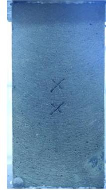
Fig. 3 A typical specimen containing two aligned X-type flaws
