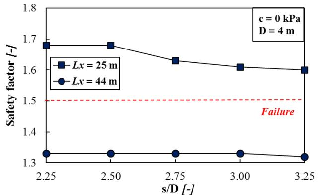
(b) Effect of pile spacing on the FoS
