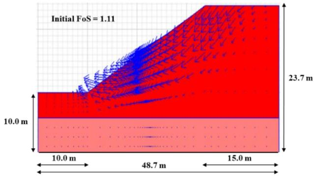
(a) Slope geometry and initial slope safety
