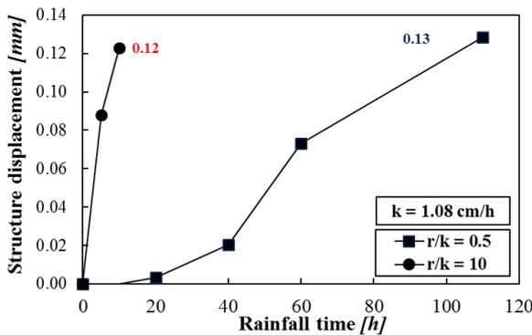
Fig. 14 Effect of rainfall on foundation displacement
