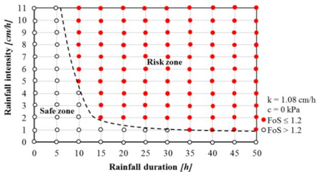
Fig. 15 Initial FoS and failure curve of the natural slope
