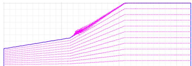
(a) Failure slope from simulation results
