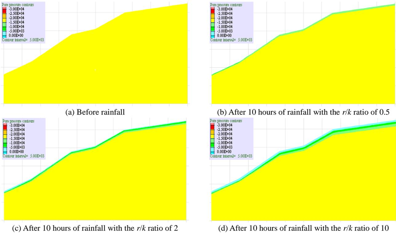
Fig. 11 Distribution of matric suction (a) before rainfall, and after 10 hours of rainfall (b) with the  $r/k$  ratio of 0.5, (c) with the  $r/k$  ratio of 2 and (d) with the  $r/k$  ratio of 10
