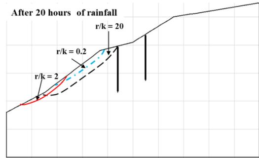
(b) Failure curve after 20 hours of rainfall
