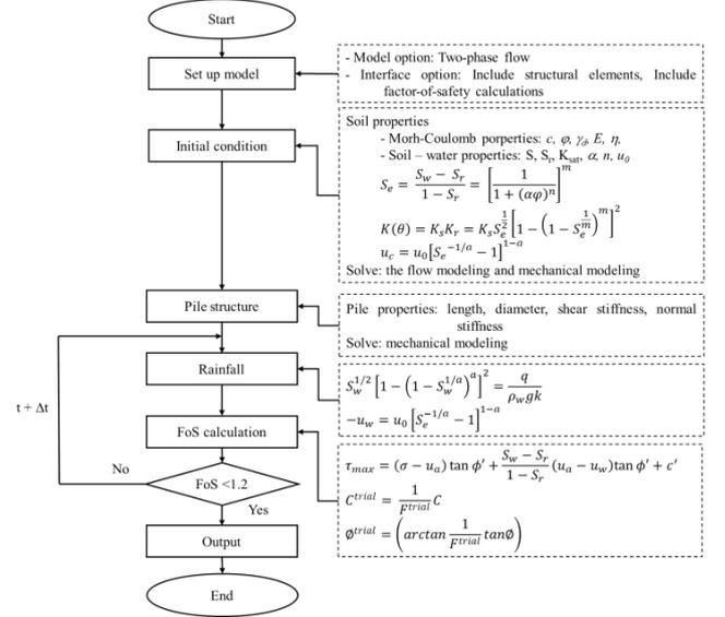
Fig. 1 Algorithm of numerical analysis on slope stability with pile foundation during rainfall
