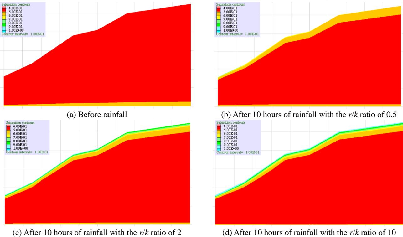
Fig. 12 Distribution of water saturation (a) before rainfall, and after 10 hours of rainfall (b) with the  $r/k$  ratio of 0.5, (c) with the  $r/k$  ratio of 2 and (d) with the  $r/k$  ratio of 10
