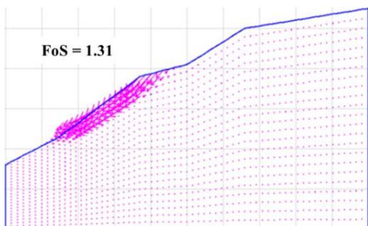
Fig. 8 Initial FoS and failure curve of the natural slope
