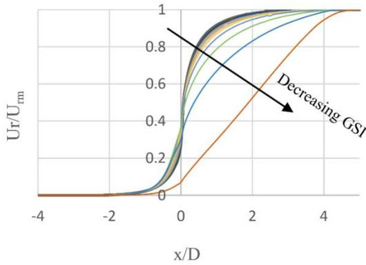
Fig. 3 Comparison of LDPs extracted from the numerical models with different GSI
