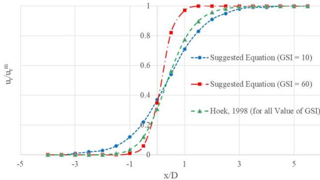
Fig. 7 Comparison of the proposed LDP at different GSI
