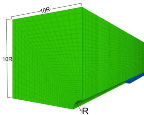
Fig. 2 Domain geometry of the developed numerical model
