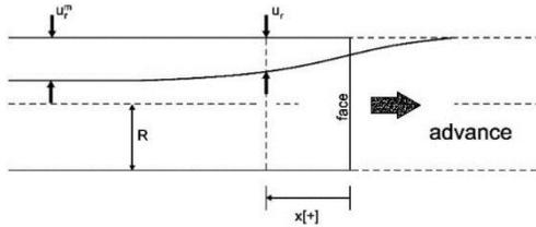
Fig. 1 Longitudinal cross-section of a tunnel
