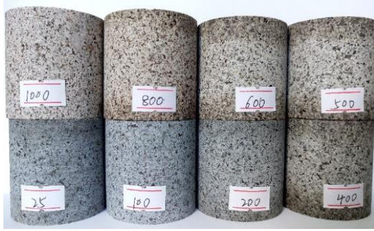
Fig. 4 Appearance of granite specimens after pretreatment
