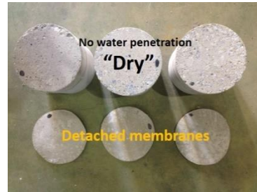
(b) Detached membranes and concrete specimens
