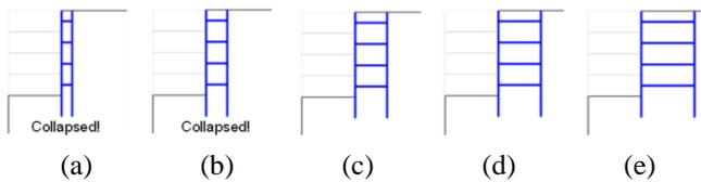
Fig. 5 Feasibility study of an earth-retaining structure using in situ soil with dual sheet piles (a) CD=1 m, (b) CD=2 m, (c) CD=3 m, (d) CD=4 m and (e) CD=5 m
