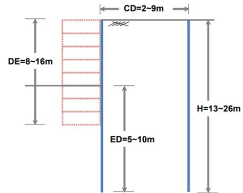
Fig. 9 Variables in numerical modeling
