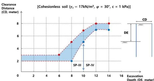
Fig. 13 Preliminary design chart for an earth-retaining structure using in situ cohesionless dry soil with dual sheet piles
