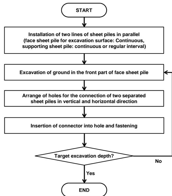
Fig. 2 Construction sequence of an earth-retaining structure using in situ soil with dual sheet piles
