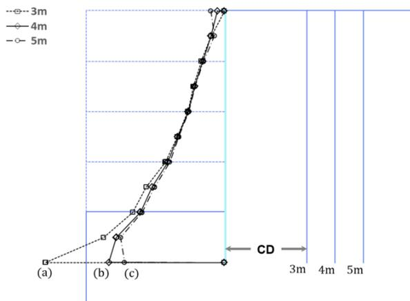
Fig. 6 Horizontal earth pressure distribution of the face sheet pile (a) CD=3 m (maximum  $\sigma'_{xx}$ = 141.6 kPa), (b) CD=4 m (maximum  $\sigma'_{xx}$ = 90.08 kPa), and (c) CD=5 m (maximum  $\sigma'_{xx}$ = 81.65 kPa)
