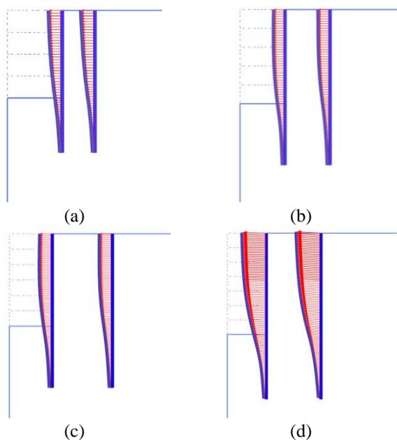
Fig. 12 Distribution of lateral displacement along sheet piles (a) Case 1 ( $\delta_{h(max)} = 0.99$  cm), (b) Case 2 ( $\delta_{h(max)} = 1.48$  cm), (c) Case 3 ( $\delta_{h(max)} = 1.76$  cm) and (d) Case 4 ( $\delta_{h(max)} = 16.1$  cm)
