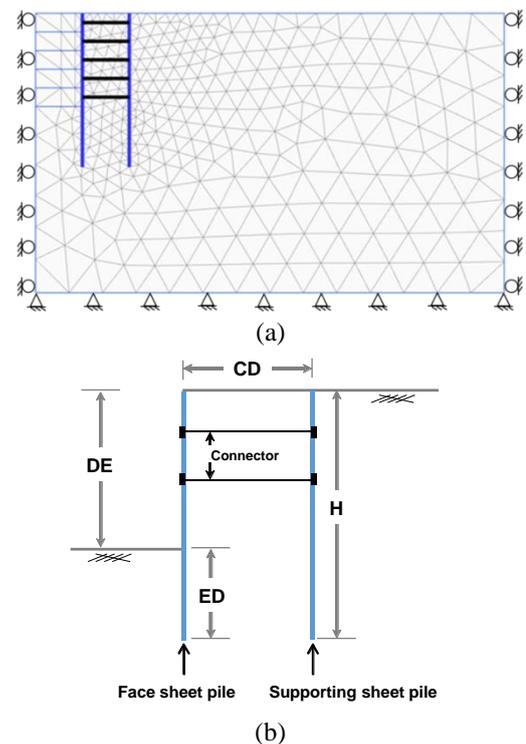
Fig. 3 Numerical model and boundary conditions for the feasibility study (a) FEM mesh and (b) Terminologies
