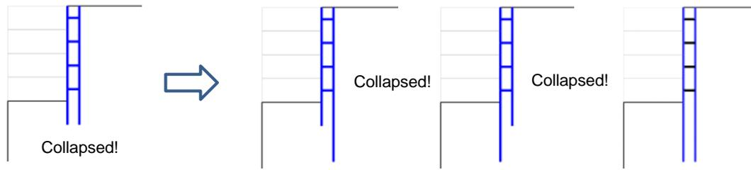
Fig. 7 Design modification for a clearance distance of 1 m
