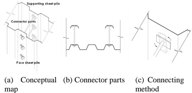
Fig. 1 Composition of an earth-retaining structure using in situ soil with dual sheet piles
