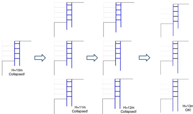
Fig. 8 Design modification for a clearance distance of 2 m
