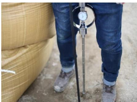
Fig. 6 Field cone penetration test
