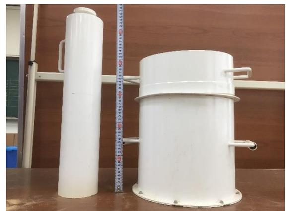
Fig. 14 Fabricated mold and rammer
