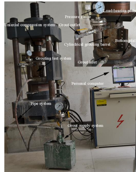
(a) Part of the penetration grouting experimental setup
