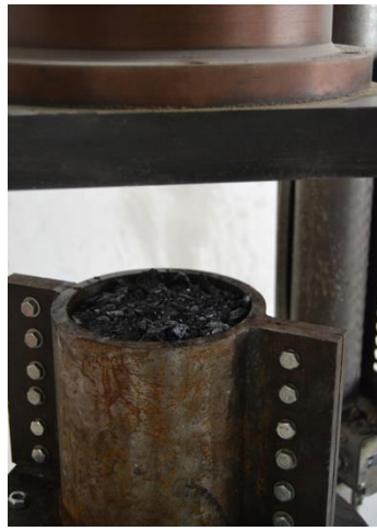
(b) Experimental specimen of crushed coal rock before grouting
