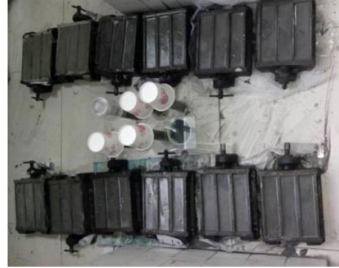
Fig. 6 Casting molds for making the specimens of the solidified grouts
