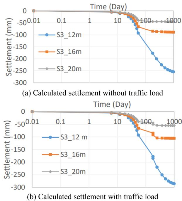
Fig. 3 Settlement-Time graphic of S3 depending on pile length
