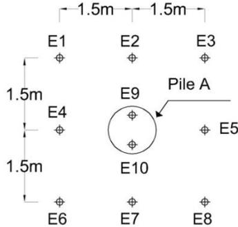
(b) Pressure measurement points around Pile A
