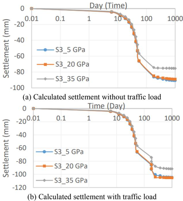
Fig. 2 Settlement-Time graphic of S3 depending on pile elasticity modulus
