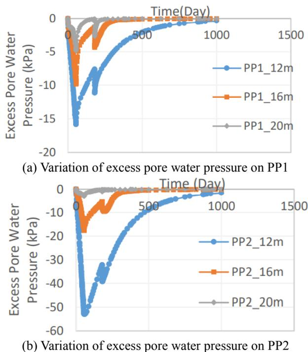
Fig. 4 Variation of excess pore water pressure with respect to time depending on pile length
