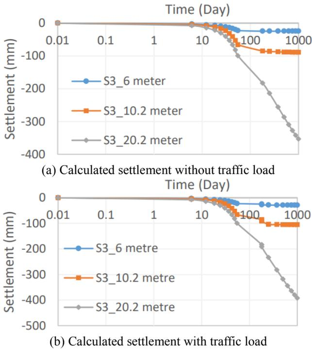
Fig. 15 Settlement variation with respect to time depending on thickness of soft soil
