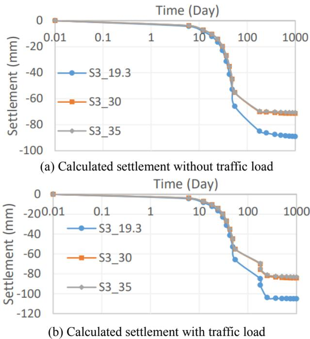
Fig. 11 Settlement variation with respect to time depending on internal angle of friction of soft soil
