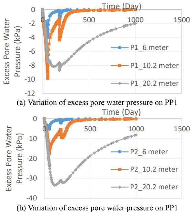
Fig. 16 Variation of excess pore water pressure with respect to time depending on thickness of soft soil
