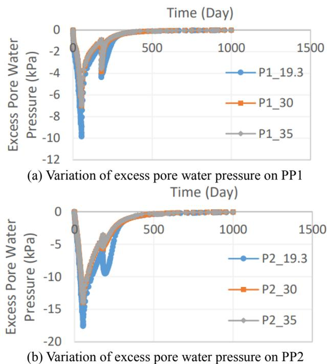
Fig. 12 Excess pore water pressure- time graphic for different internal angle of friction of soft soil
