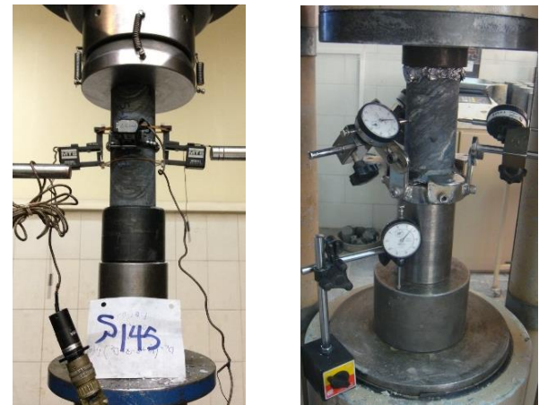
(a) Clip and chain-type extensometers (b) Dial gauges
